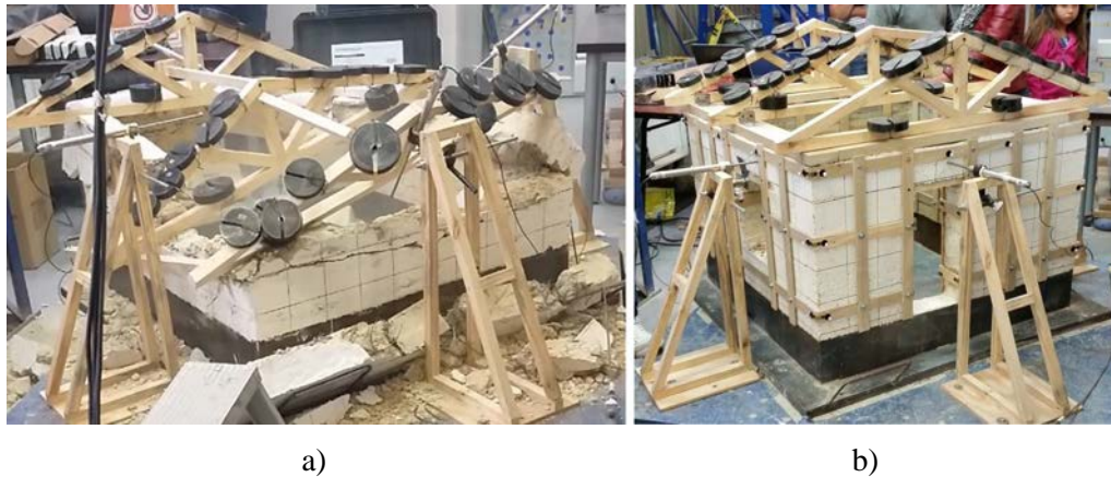
Fig. 7 – Global behaviour of: a) unreinforced model after the test, and b) reinforced model after the test
