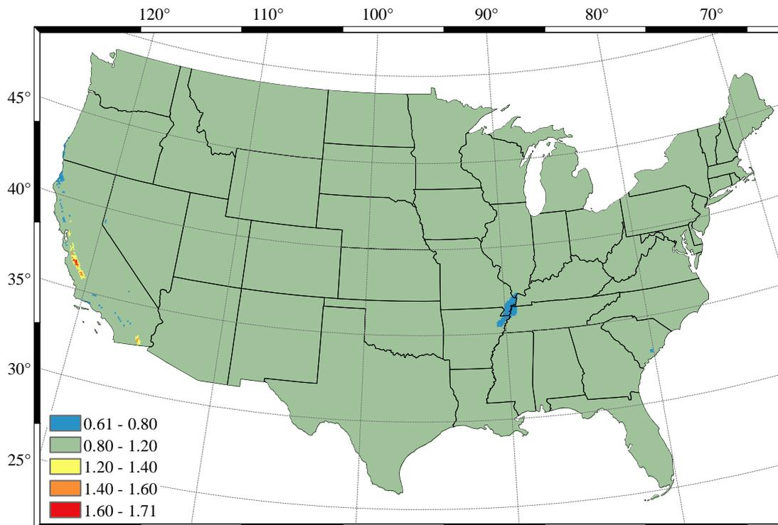
**Fig. 6** – Ratios of the alternative, purely probabilistic  $MCE_R$  ground motions (from Fig. 5) divided by the  $MCE_R$  ground motions mapped in the 2015 NEHRP Provisions, for the 0.2-second spectral response accelerations shown in other figures of this paper. The ratios for the 1.0-second spectral response accelerations are similar. Please see Fig. 9 for a zoomed-in map covering California.
