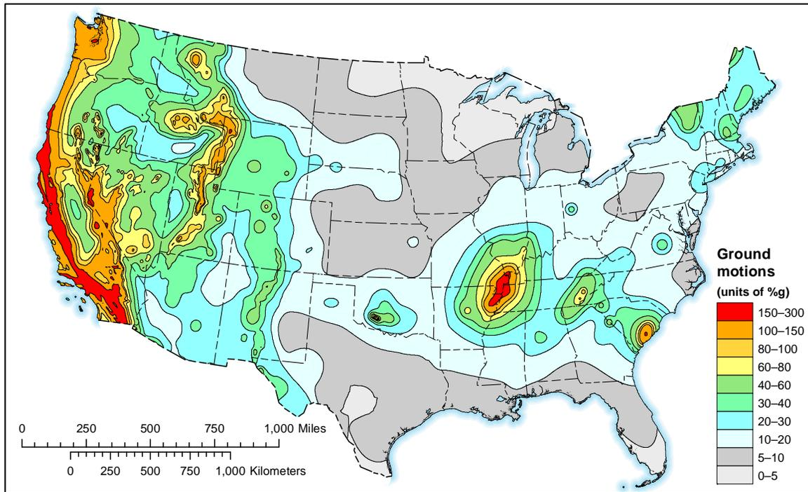
**Fig. 5** – Alternative, purely probabilistic  $MCE_R$  ground motion map at a spectral period of 0.2 seconds.
