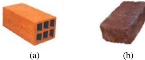
Fig. 1 Horizontal hollow brick (a) and handmade solid brick (b)
