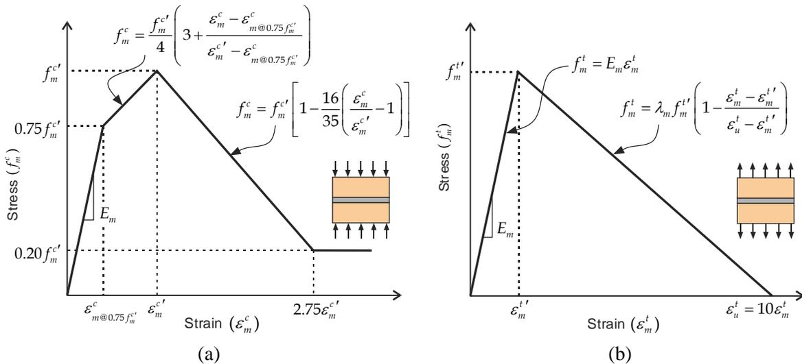
Fig. 3 – Material model of masonry specified in finite element analyses: a) compressive stress-strain curve, and b) tensile stress-strain curve
