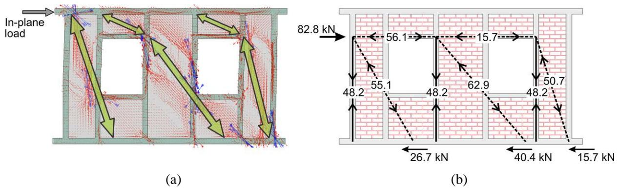
Fig. 9 – Wall W4: (a) principal stress vector plots, and (b) strut-and-tie model
