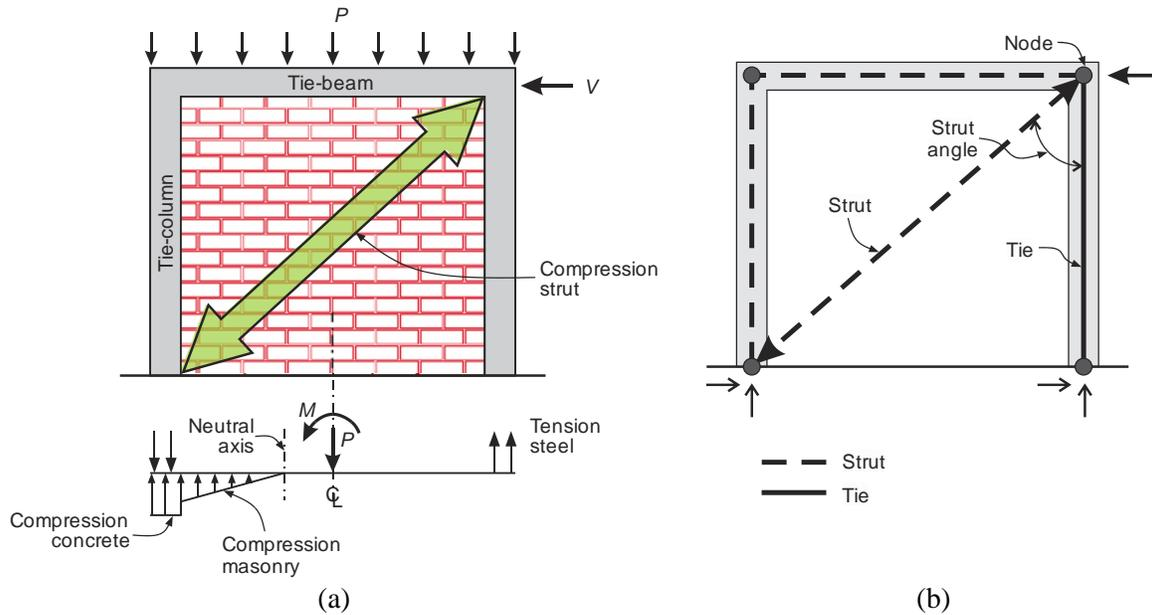
Fig. 7 – (a) Internal force distribution in a confined masonry wall panel subjected to combined axial load and bending (redrawn from Meli et al. [23]), and (b) a possible strut-and-tie model for confined masonry wall
