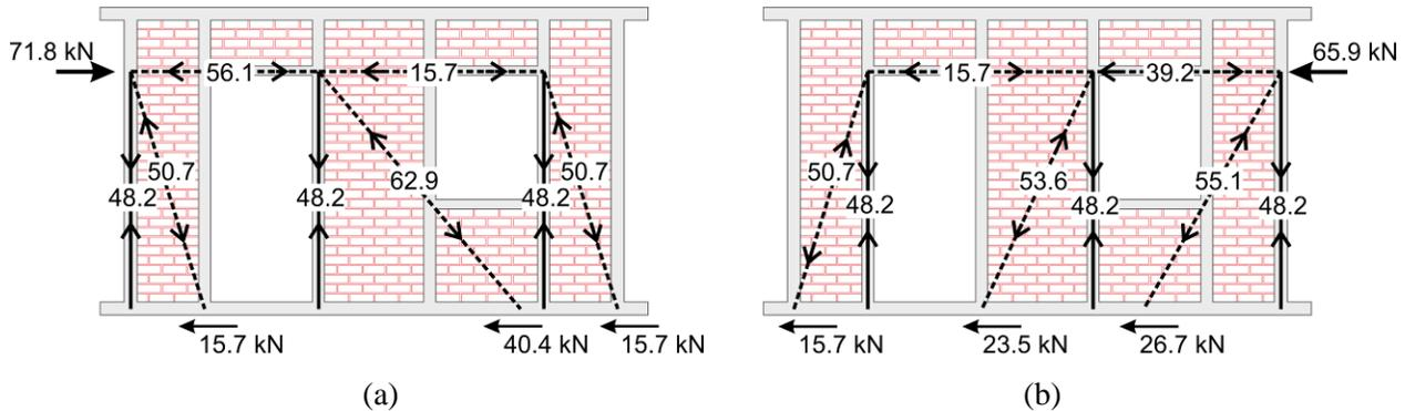
Fig. 11 – Strut-and-tie model for wall W6: (a) push direction, and (b) pull direction
