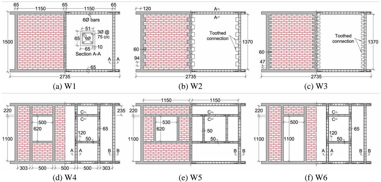
Fig. 1 – (a) – (f) Details of confined masonry wall specimens
