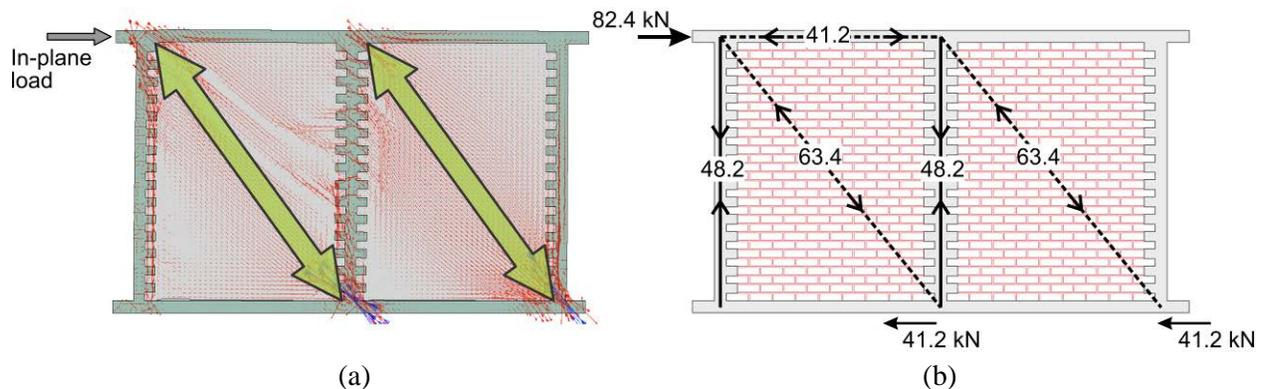
Fig. 8 – Wall SCFT: (a) principal stress vector plots, and (b) strut-and-tie model
