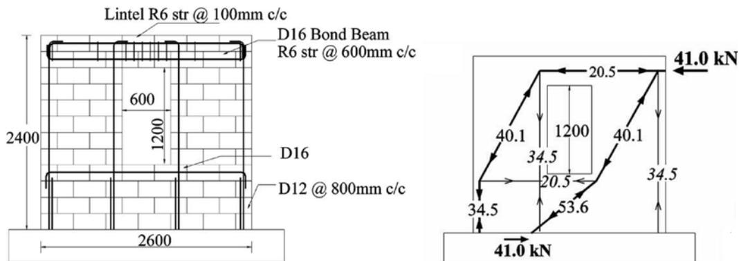
Fig. 6 – Strut-and-tie model for the reinforced masonry wall with an opening [19]
