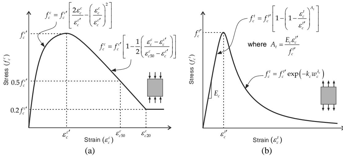
Fig. 4 – Material model of concrete specified in finite element analyses: a) compressive stress-strain curve, and b) tensile stress-strain curve
