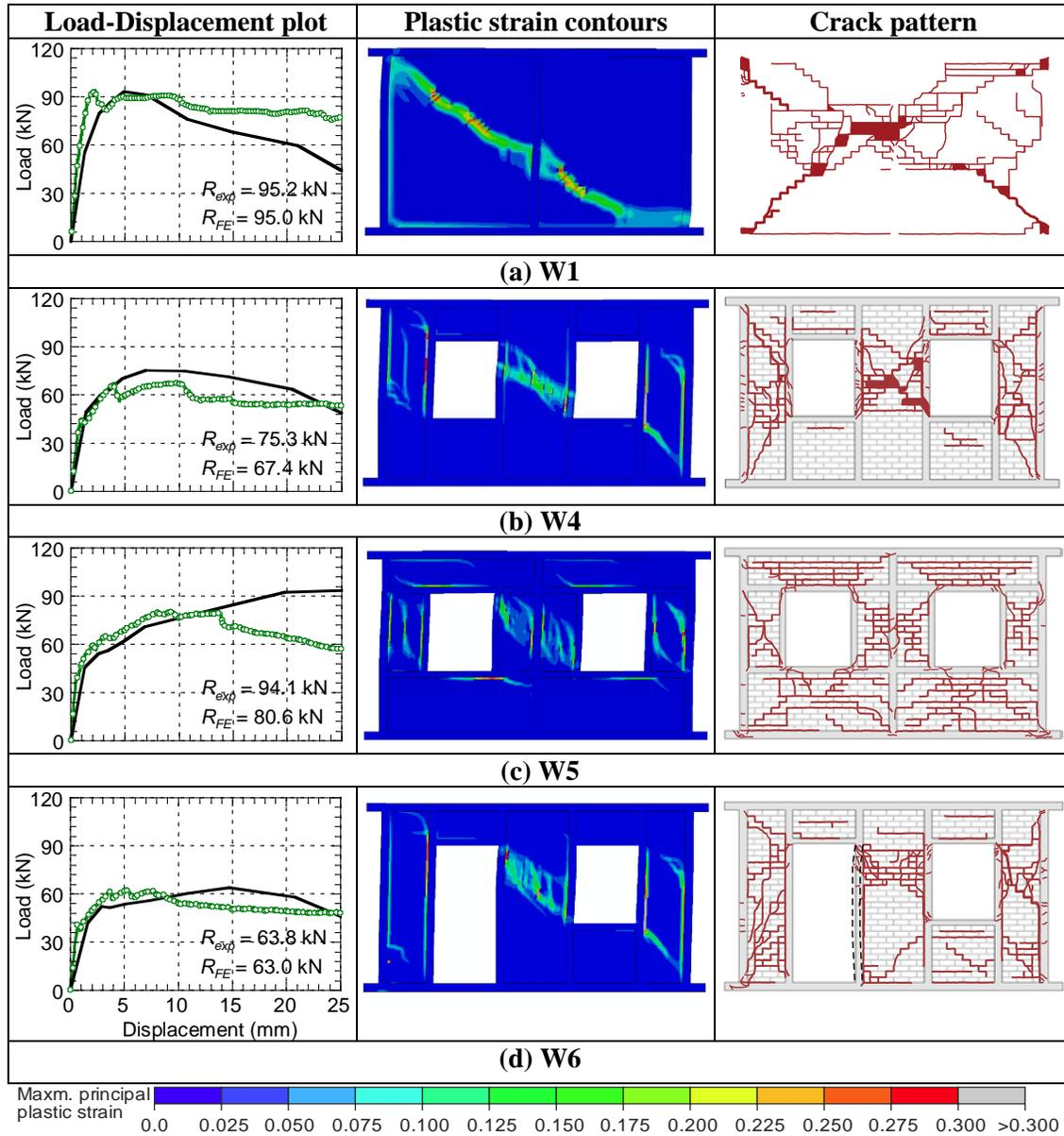
Fig. 5 – Comparison of load-displacement curve and crack patterns obtained from experiments and FE simulation for confined masonry walls: (a) W1, (b) W4, (c) W5, and (d) W6
