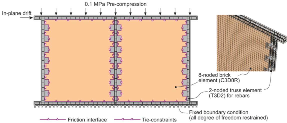
Fig. 2 – Schematic diagram of a typical wall illustrating various elements used in the finite element analyses
