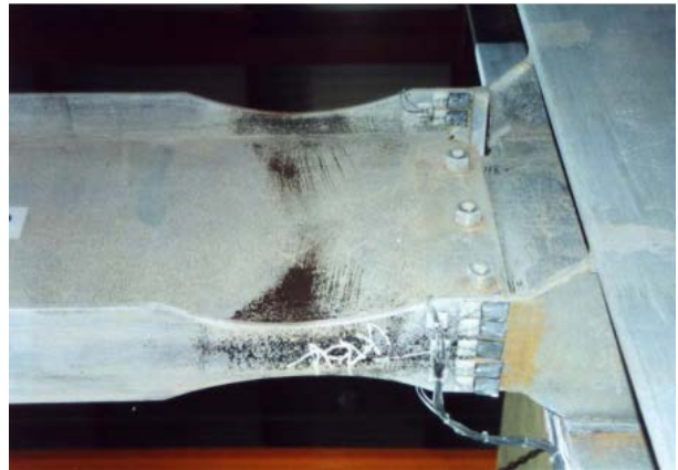
(b) Beam Damage at Plastic Rotation of about 0.01 Radian (Pictures from Gilton et al. [7])
