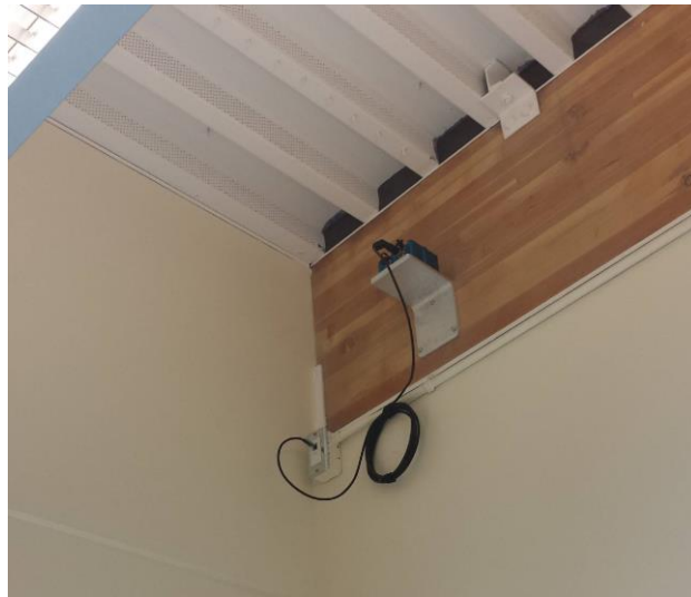
Fig. 8 – Example strong motion sensor in school
