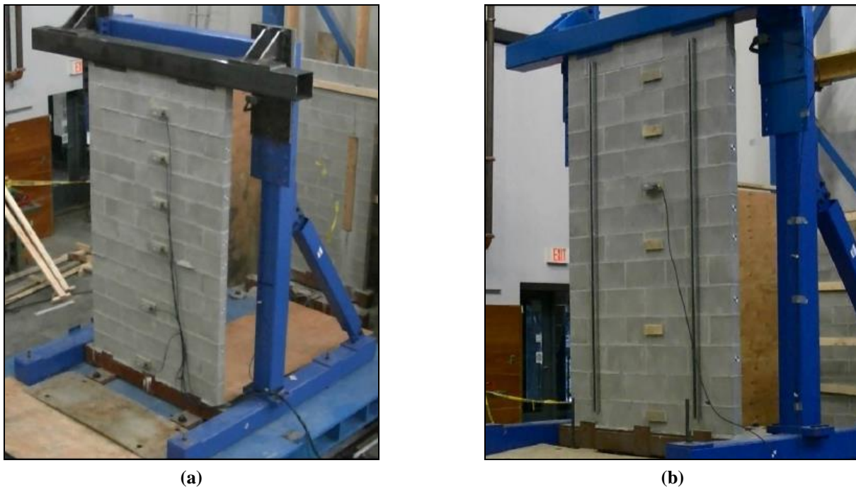
Fig. 7 – Out-of-plane URM specimens: a) bare 4’ concrete block wall b) vertical Unistrut® retrofit
