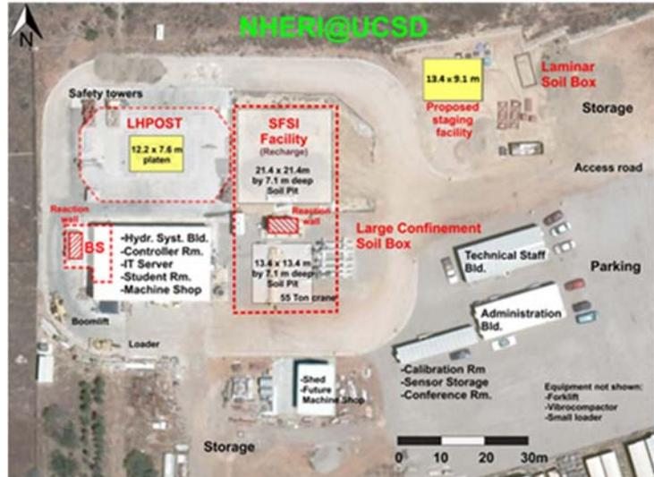
Fig. 1 – Plan view of the Englekirk Structural Engineering Center (ESEC).
