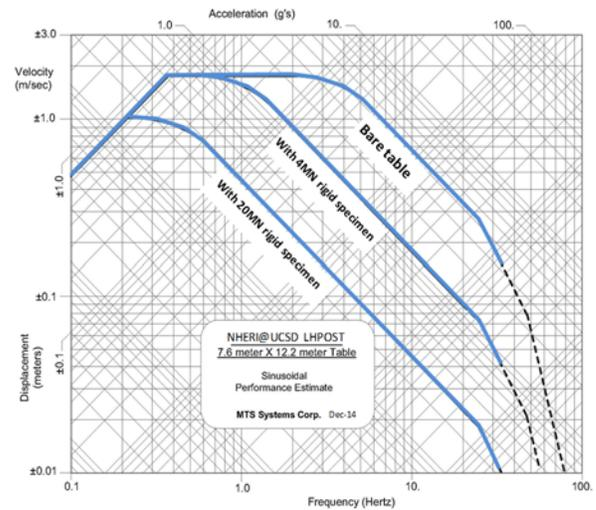
Fig. 4 – LHPOST performance specifications
