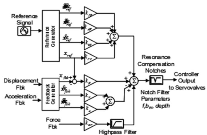
Fig. 7 – Conceptual representation of MTS TVC controller.
