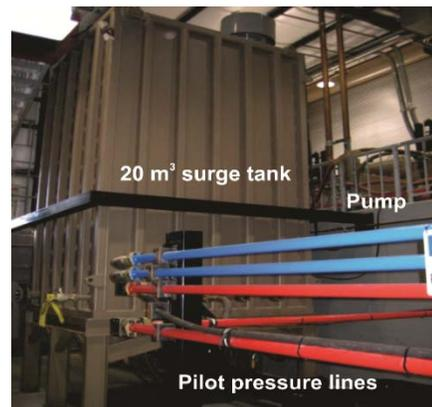
Fig. 6 – Oil surge tank and pilot pressure lines
