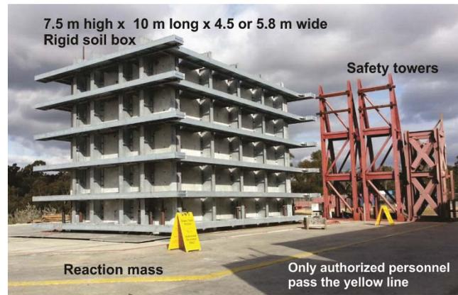
Fig. 9 – Large soil confinement box installed atop of the shake table platen, safety towers and safe area.
