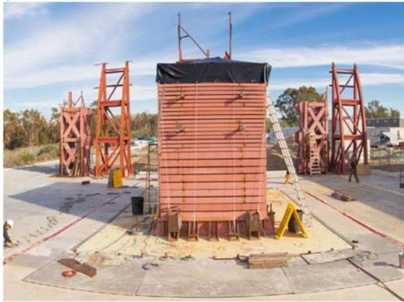
Fig. 8 – Large laminar soil box installed atop of the shake table platen
