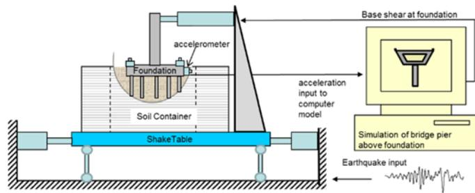
(b) Bridge pier including soil-structure-interaction effects
