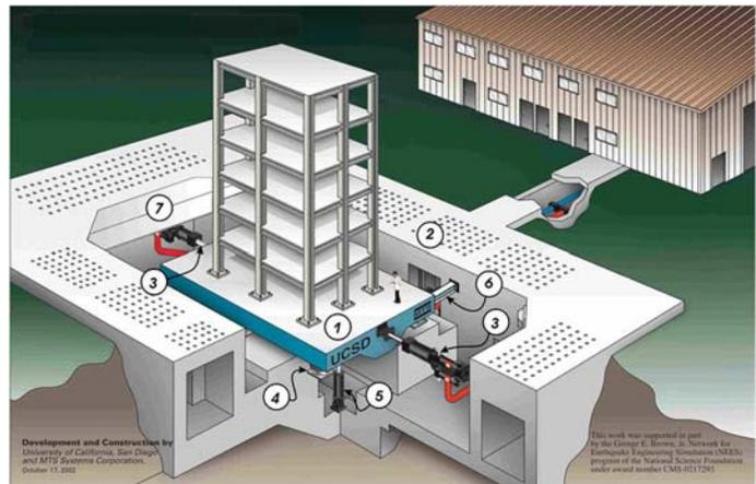
Fig. 3 – Schematic representation of the NHERI@UCSD Shake Table.
