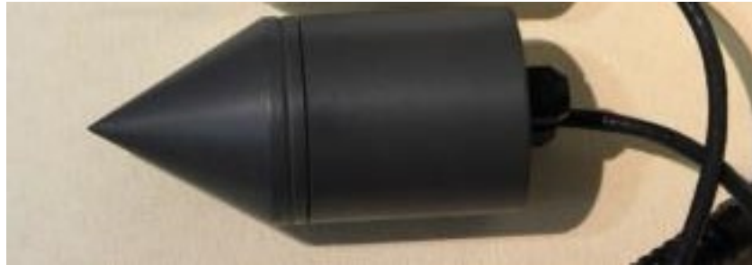
Figure 3. Tetra sensor in downhole configuration
