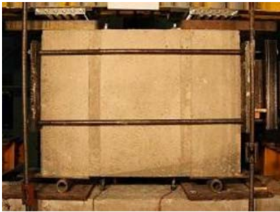
a) Seismic bars touching the PVC tubes of the diaphragm, specimen WD2
