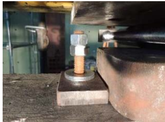
a) Uplift of the seismic bar nuts, specimen WD2
