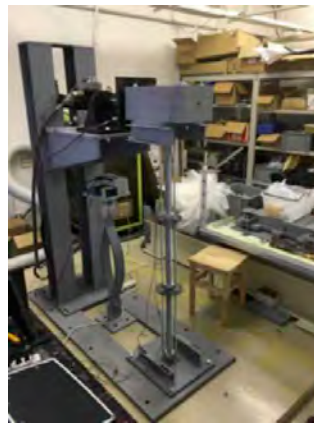
Figure 12 1/15 scale experimental model of aerogenerator
