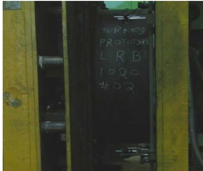
Fig. 3– Tension testing on 1020LRB190 Unit
