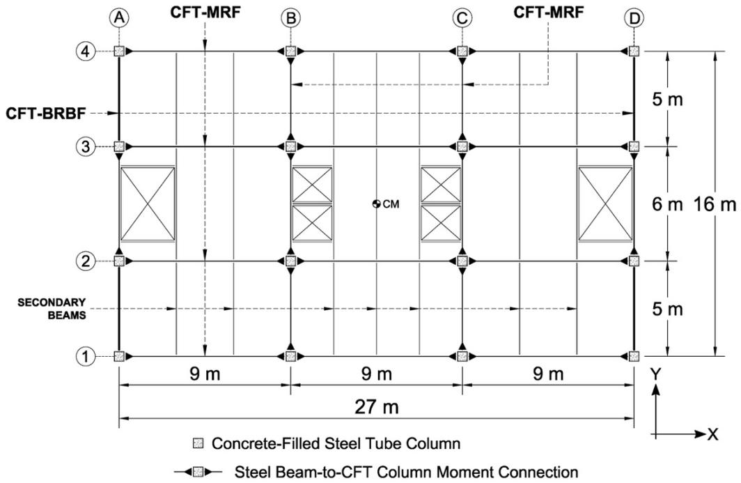
Fig. 1 – Typical floor plan of the prototype building
