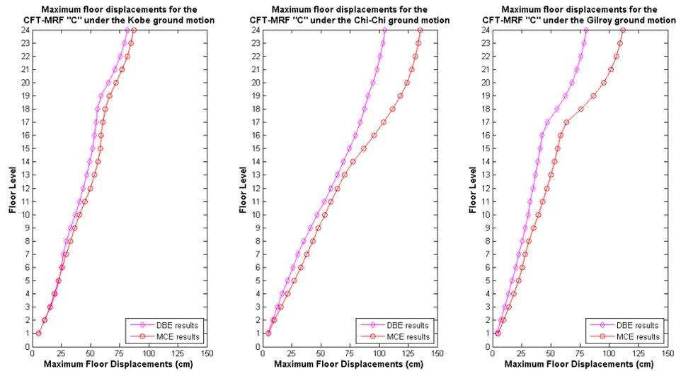
Fig. 9 – Maximum floor displacements for the CMFR under Kobe, Chi-Chi and Gilroy ground motions
