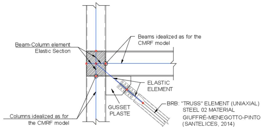
Fig. 5 – OpenSees nonlinear analytical model for the BRBF
