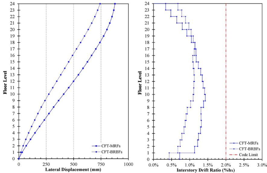
Fig. 3 – Story displacement and interstory drift ratio distribution along prototype building height
