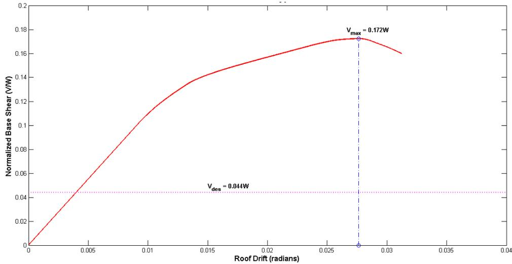
Fig. 6 – Results of the Non Linear Static Analysis (Pushover) – X - Direction (CMRF)
