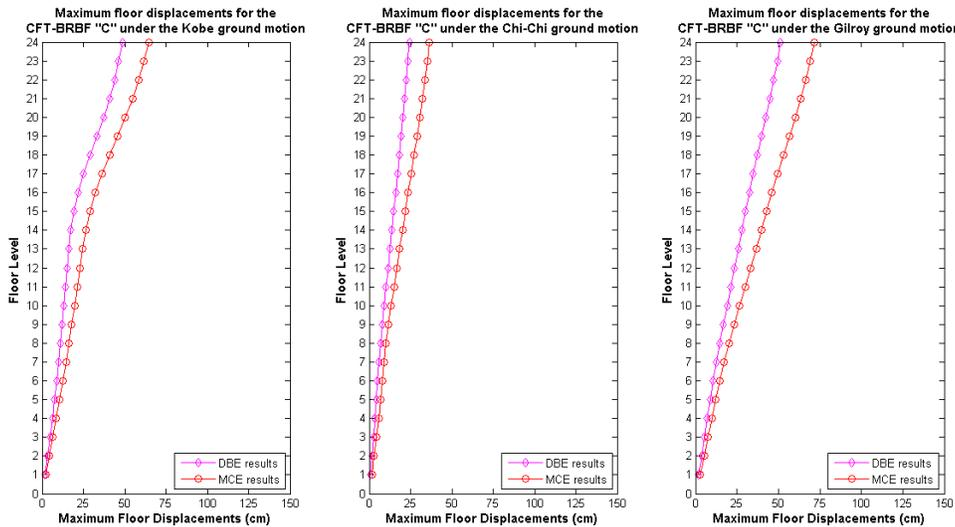
Fig. 10 – Maximum floor displacements for the BRBF under Kobe, Chi-Chi and Gilroy ground motions
