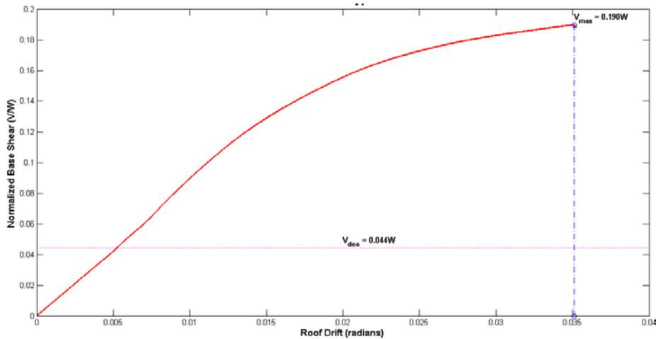
Fig. 7 – Results of the Non Linear Static Analysis (Pushover) – Y - Direction (BRBF)
