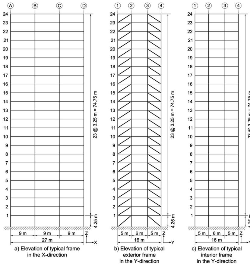
Fig. 2 – Elevation of the typical frames in the X and Y direction
