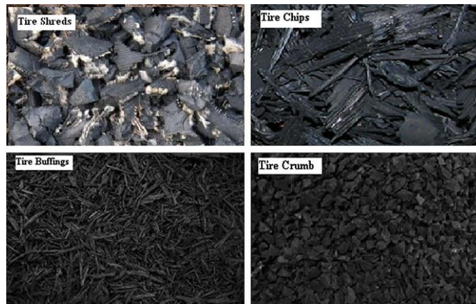
Fig. 1- Typical shapes of different processed tire wastes (not to scale) [5].
