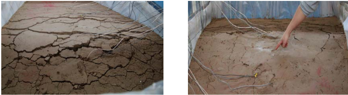
Fig. 6 – Failure of the slope model with 10mm rainfall in the shaking table tests (left:1000gal; right: 700 gal)
