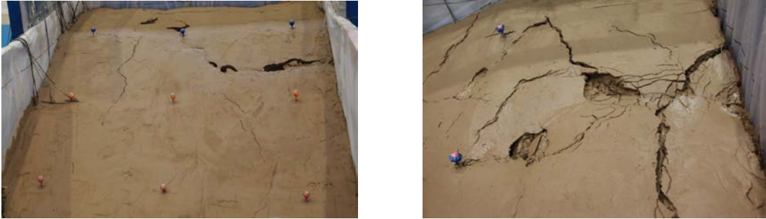
Fig. 8 – Failures of the slope model with 100mm rainfall (left) and then under the loading of 400gal (right)
