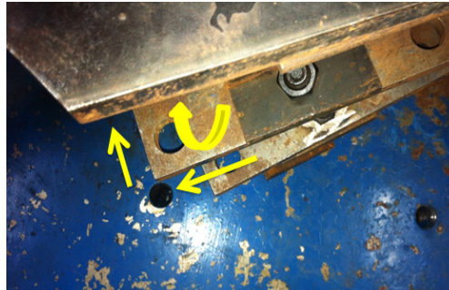
Fig. 30 – Relative movement of upper and lower steel plates
