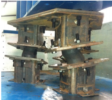
Fig. 29 – 3DRSI vertical deformation
