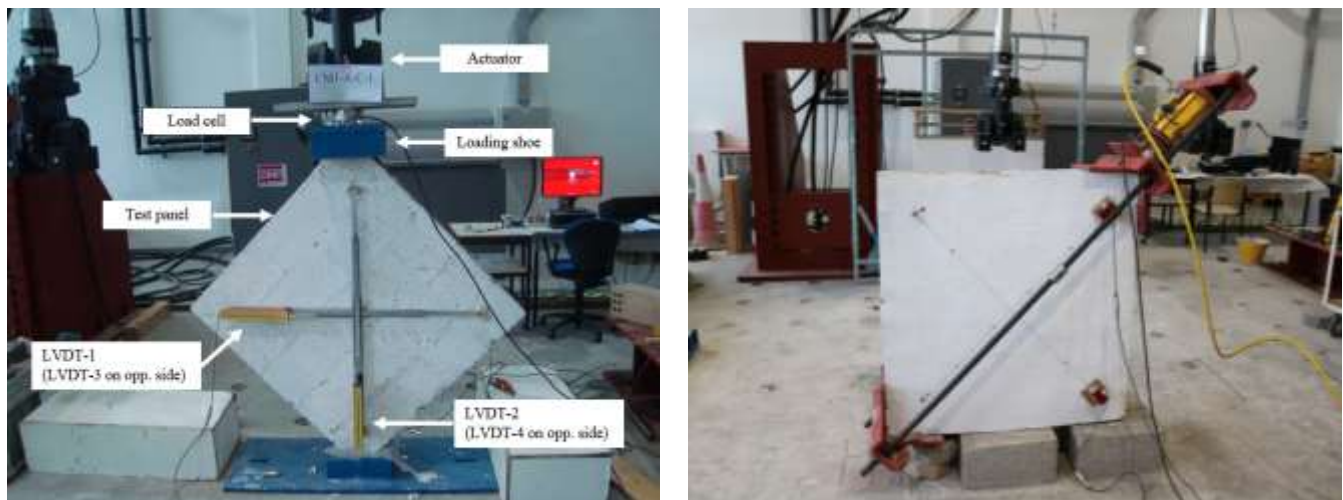
(a) Test setup for As-built specimen
