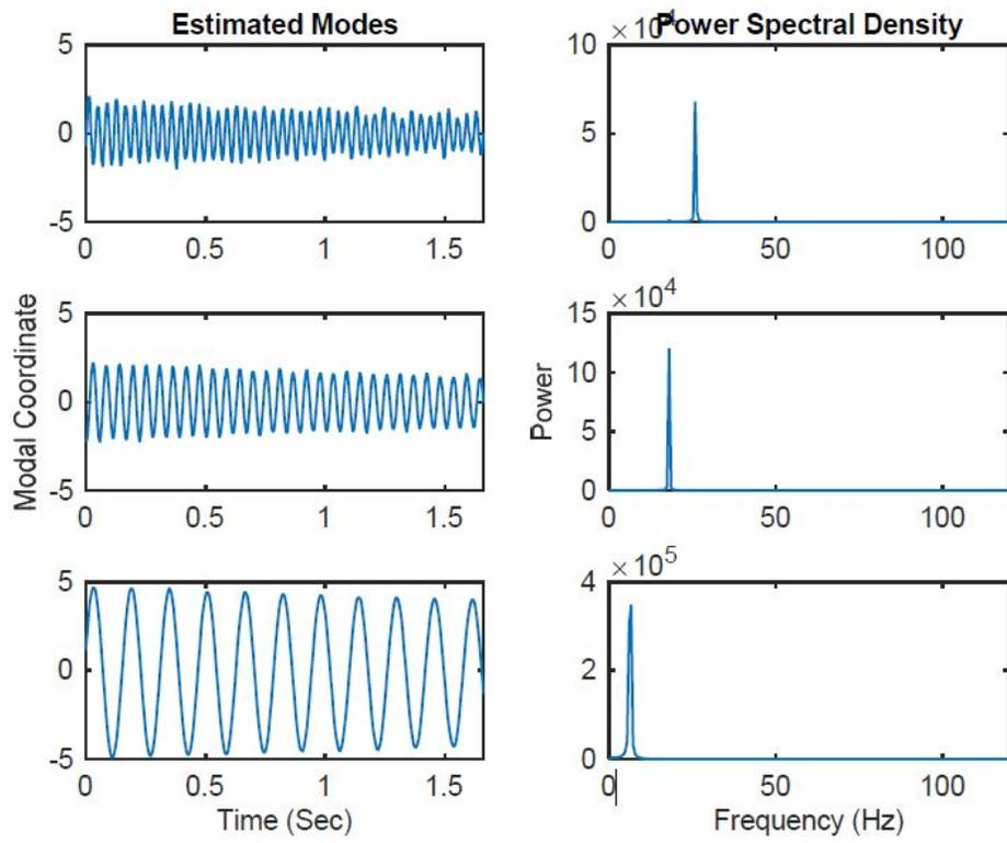
Fig. 1 – Complexity Pursuit (CP) estimated modal coordinates and their power spectral density from the video measurement of the vibrating building structure.
