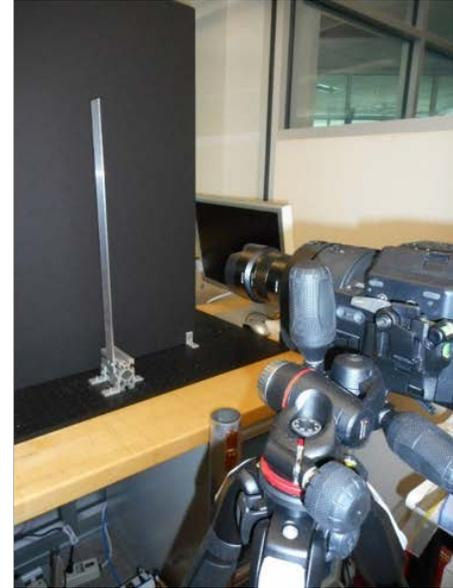
Fig. 1 – Experimental Setup of the 3-story building structure and the cantilever beam, both excited by the impact force.
