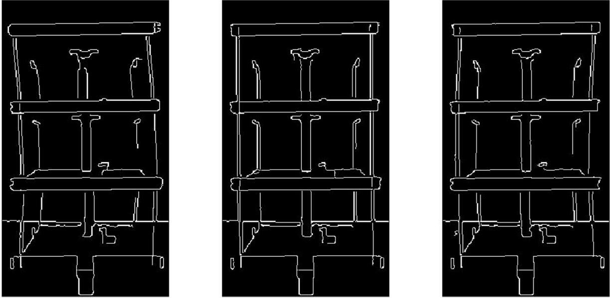
Fig. 3 – A few frames from the blindly-separated, motion magnified Video (**Mode 2**) (**first row**) of the building structure (excited by an impact) and their corresponding full-field, very high spatial (pixel) resolution mode shapes (**second row**) by conducting the edge detection. For the complete video demos of the experimental results (including other modes), see at <http://www.lanl.gov/projects/national-security-education-center/engineering/research-projects/blind-modal-id.php>.
