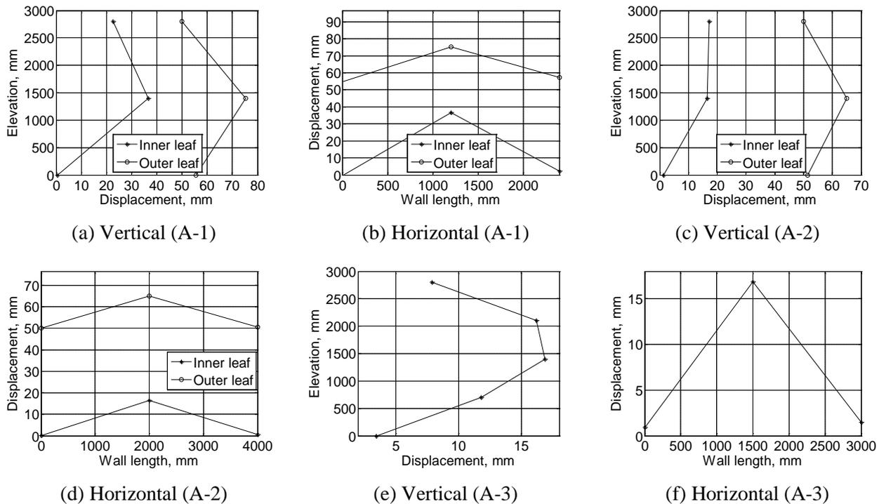
Figure 10: Deflected profile of walls in Building A
