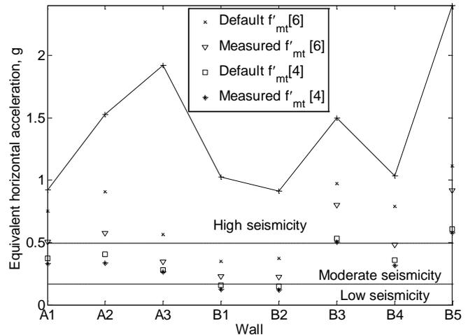
Figure 12: Comparison between the measured and predicted wall strength and the range of seismic demand for regions with different seismicity
