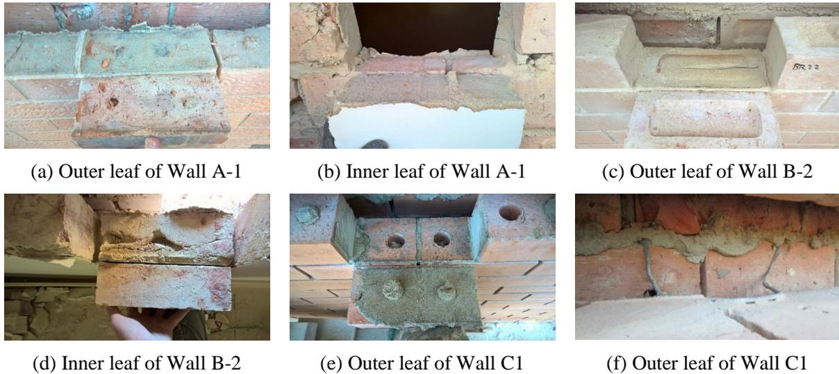
Figure 2: Brick types, failure pattern in bond wrench tests, and typical cavity tie
