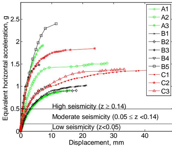
Figure 11: Recorded force-displacement data for all walls and comparison with estimated seismic demand
