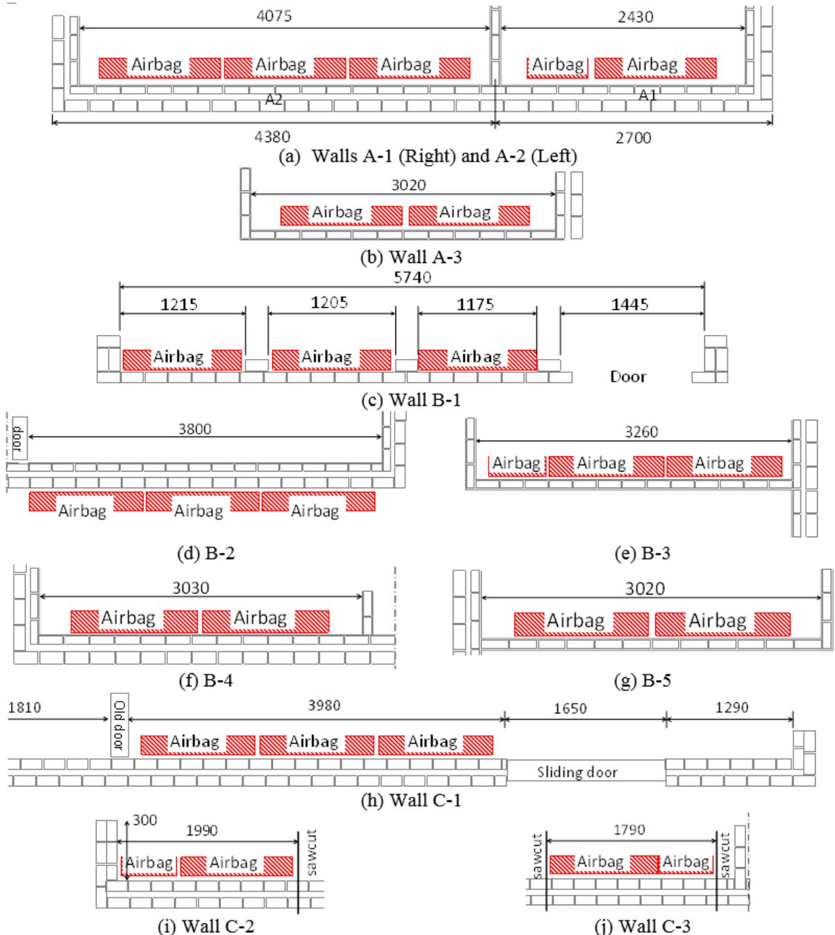
Figure 5: Plan view showing support configuration and direction of airbag loading
