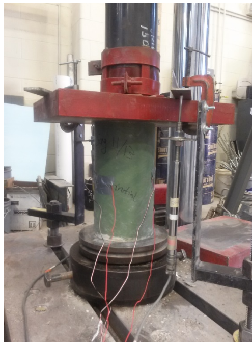
Fig. 3 - Setup for the compression test on CFFT cylinders
