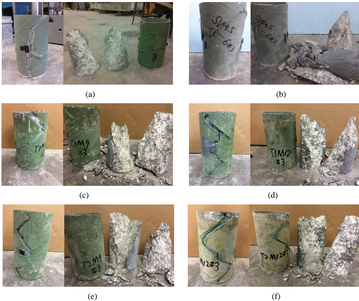
Fig. 5 - Failure modes of the outer FRP tubes and core concrete for several CFFT specimens: (a) CFFT_UC#3; (b) CFFT_T1M6#3; (c) CFFT_T1M9#3; (d) CFFT_T1M12#3; (e) CFFT_T2M9#3; (f) CFFT_T2M12#3
