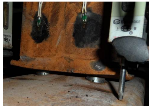
Fig.15 – The deformation of the connection
