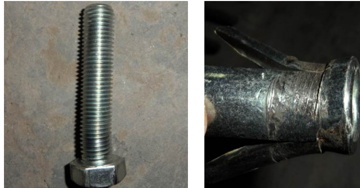
Fig.12 – The deformation of blind bolt
