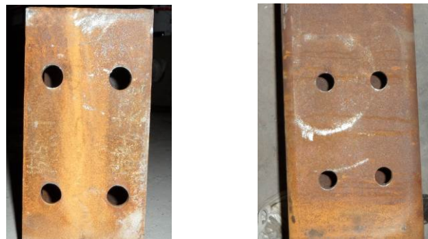
(1) bolt opening on the end plate (2) bolt opening on the column wall
