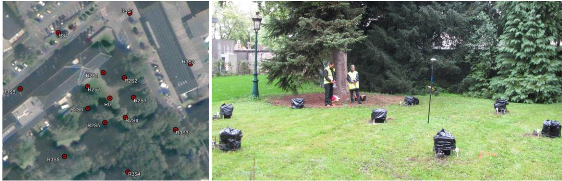
Figure 3 – Left: location of the 15 broadband seismometers on a double circle geometry (here, with radii of 15 and 45 m) at the OGAP station. Right: inner circle (radius = 5 m) of an AVA acquisition near the OGAP station.
