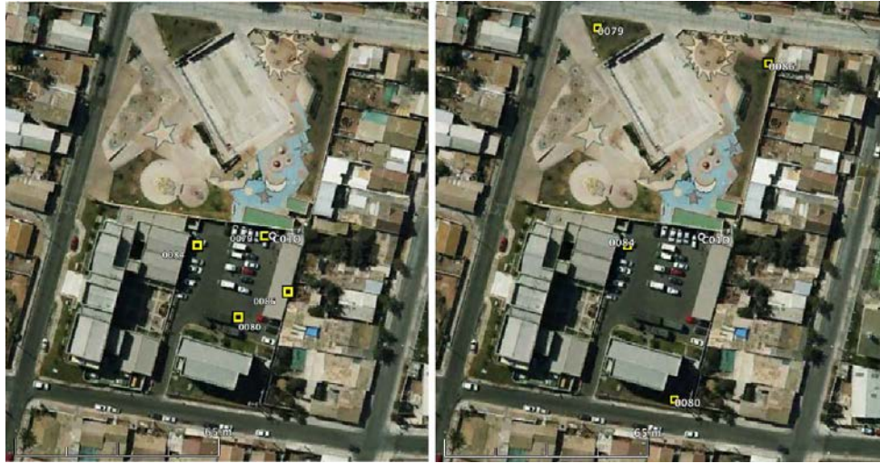
Fig. 3 – Google Earth maps showing examples of the geometry used in the array measurements, these come from the C010 station: each yellow square shows the location of a geophone and the white circle represents the strong-motion station.
