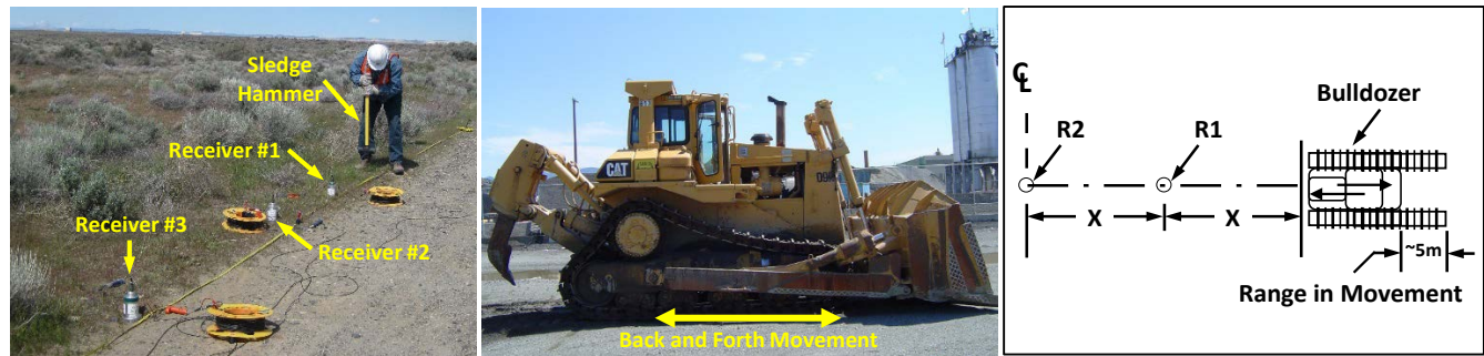
(a) Sledge hammer often used at short (< 5 m) receiver spacings (b) Bulldozer used as a high-energy source for moderate (< 75 m) profiling (c) Typical back-and-forth movement of bulldozer
