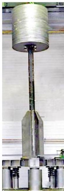
Fig. 9 – Model of switch based on one spring device
