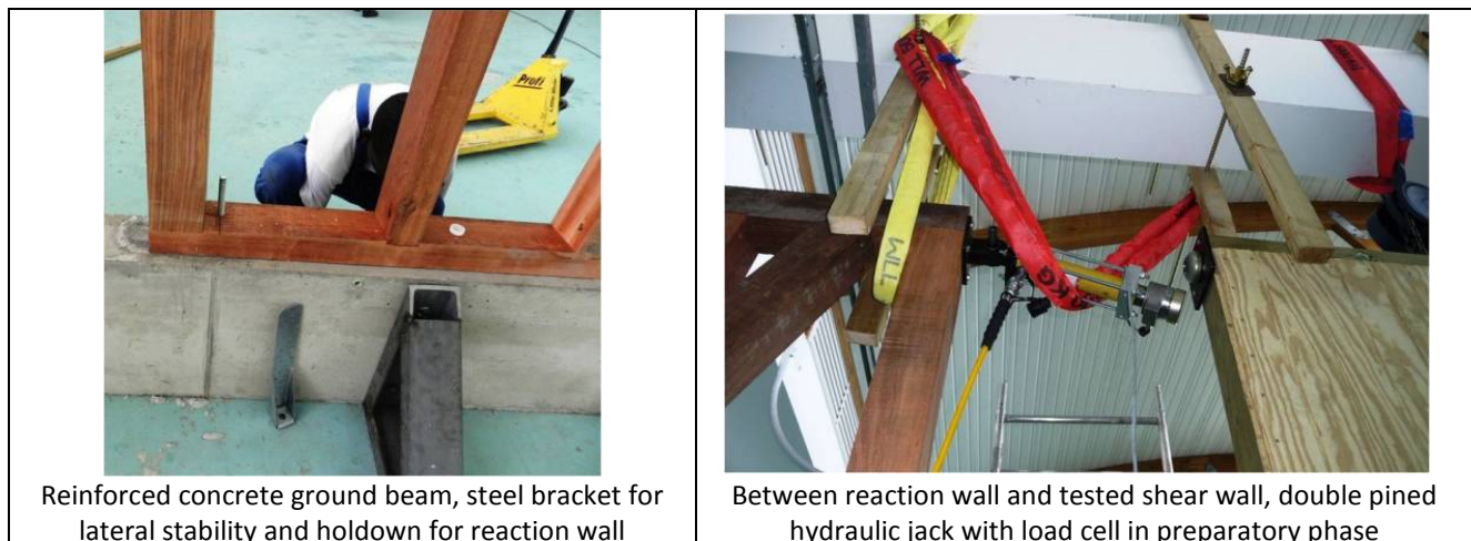
Fig 2. Illustrations of experimental setup
