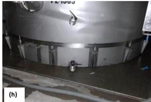
Diamond shaped buckling
