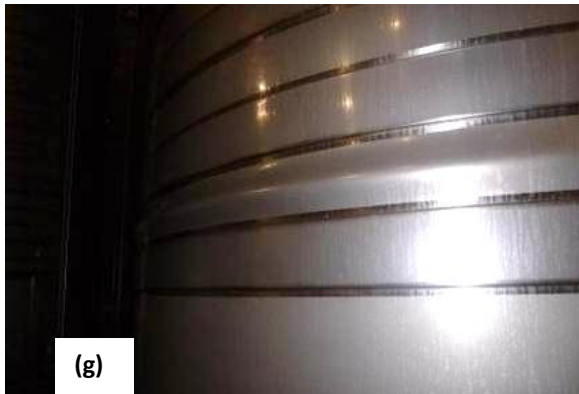
Elephant's foot buckling of tank
