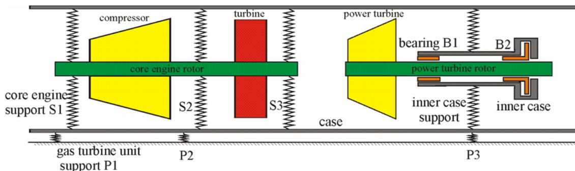
Fig. 1 – Gas turbine unit rotors model
