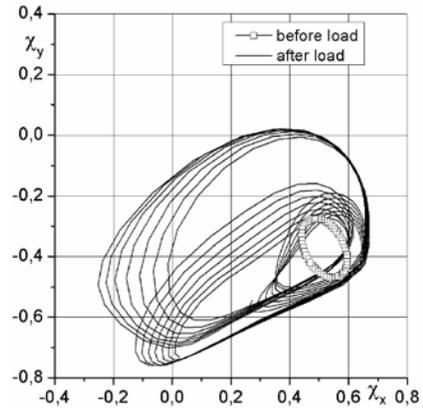
b) rotor orbits in bearing B1 for excitation frequency  $f = 18$  Hz
