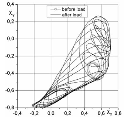
d) rotor orbits in bearing B1 for excitation frequency  $f = 16$  Hz
