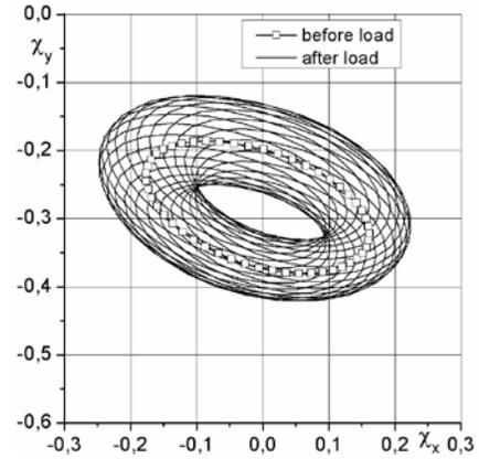
b) rotor orbits in bearing B1 for excitation frequency  $f = 18$  Hz (axial excitation)
