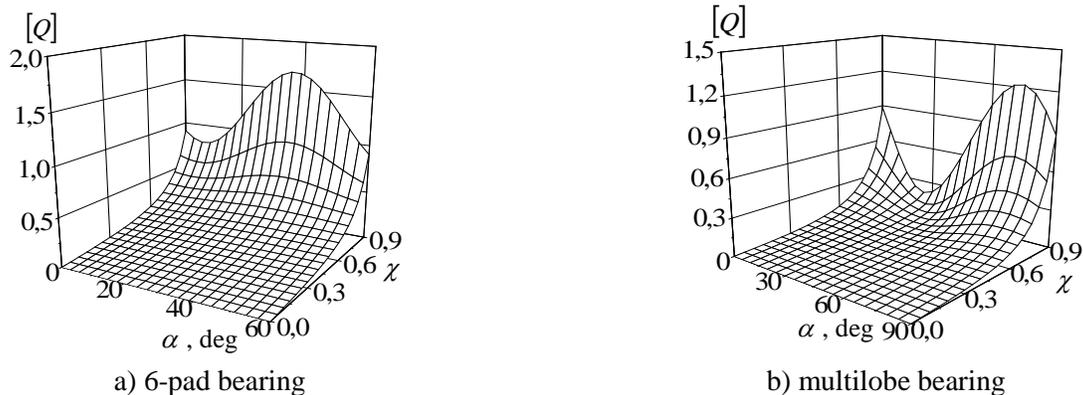
Fig. 4 – Bearing carrying force versus  $\alpha$  and  $\chi$
