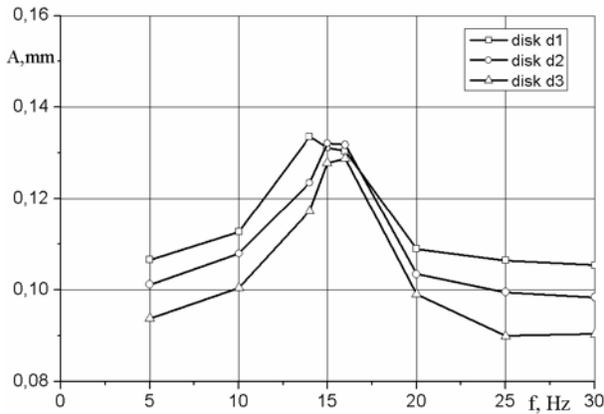
c) maximal relative change of gap in gasdynamic path at lateral excitation
