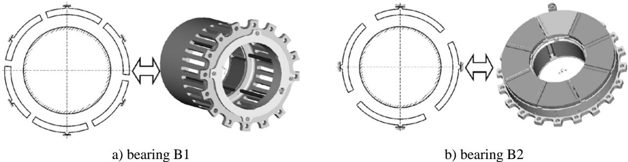
Fig. 3 – Hydrodynamic pad bearings
