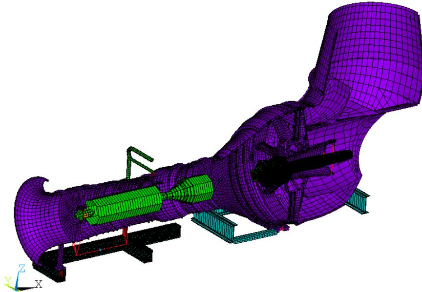
Fig. 2 – Stationary gas turbine unit shell-beam finite element model
