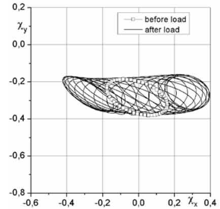
d) rotor orbits in bearing B1 for excitation frequency  $f = 16$  Hz (lateral excitation)
