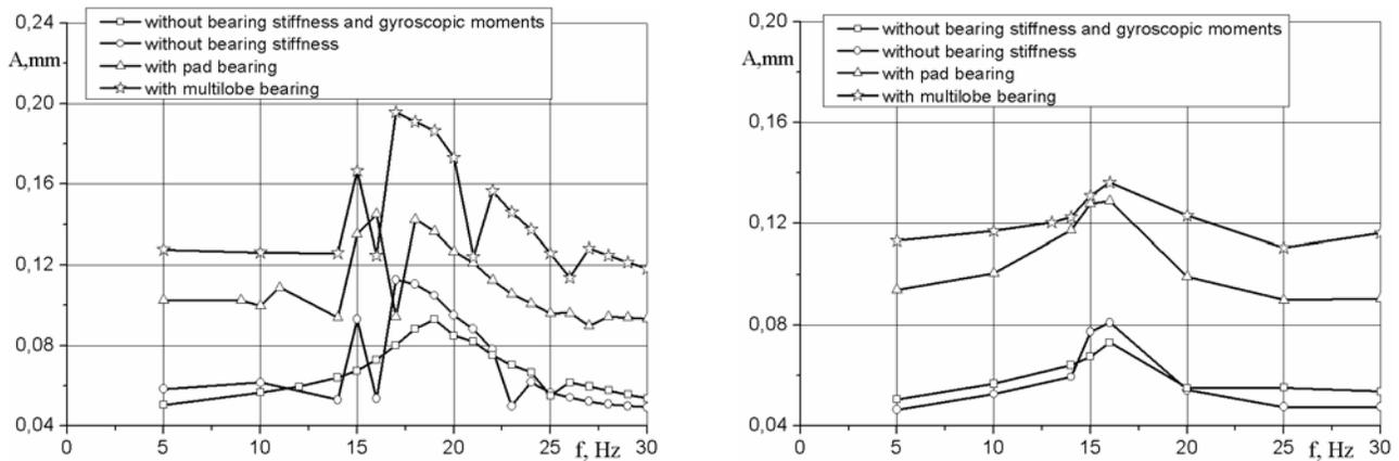
a) maximal relative change of gap in gasdynamic path at axial excitation      b) maximal relative change of gap in gasdynamic path at lateral excitation
