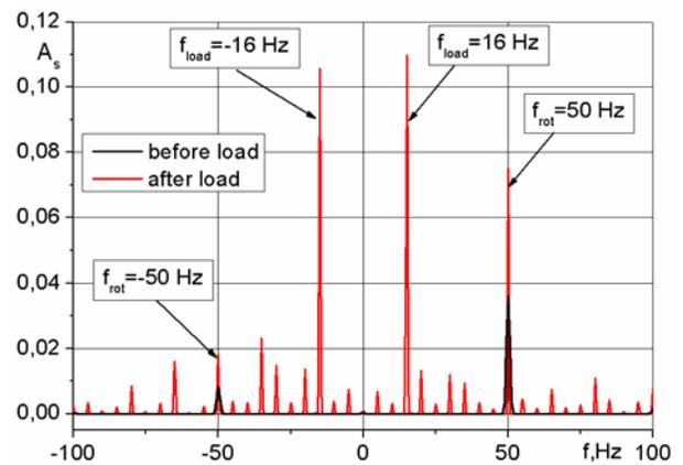
f) full spectrum of orbit in bearing B1 for excitation frequency  $f = 16$  Hz (lateral excitation)
