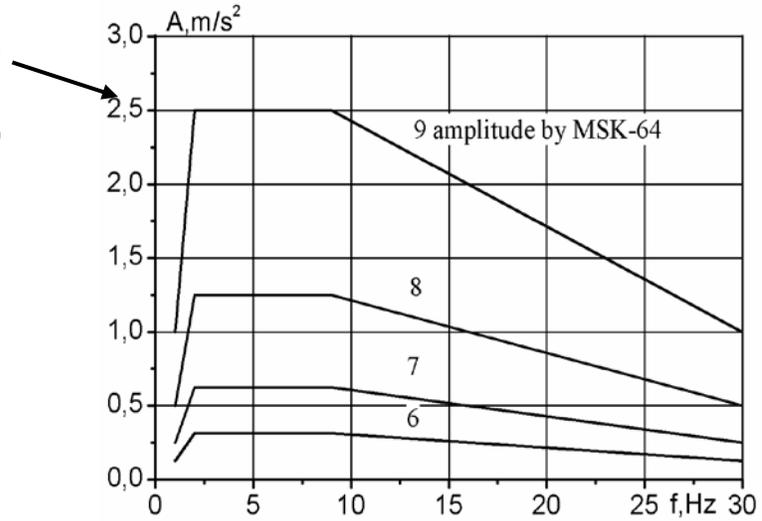
c) foundations accelerations for different earthquake amplitude by MSK-64 [1]
