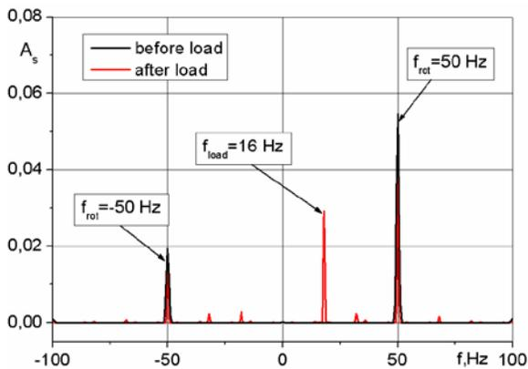
e) full spectrum of orbit in bearing B1 for excitation frequency  $f = 18$  Hz (axial excitation)
