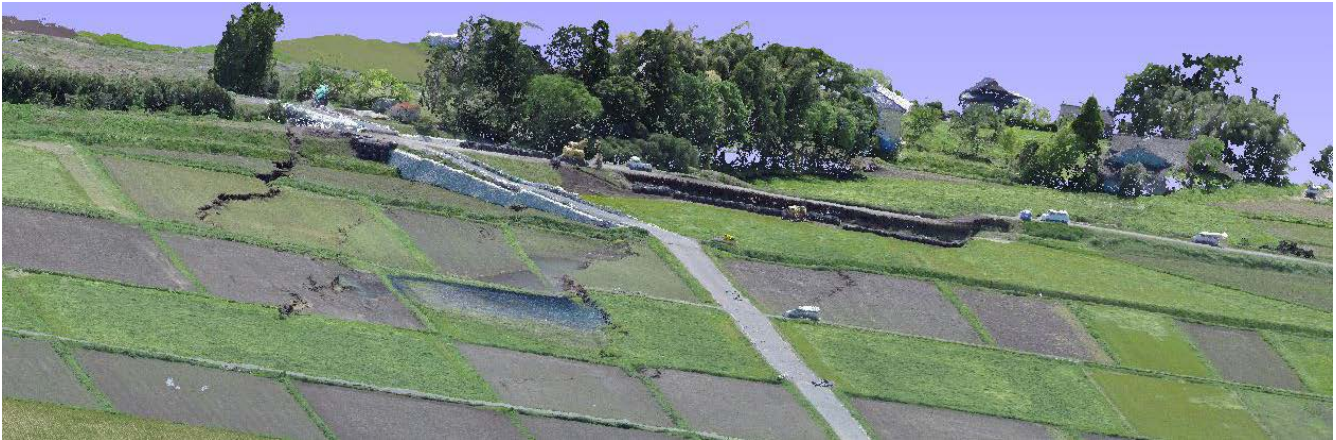
Fig. 6 Portion of the depression zone shown in the 3D point cloud model developed from UAV.
