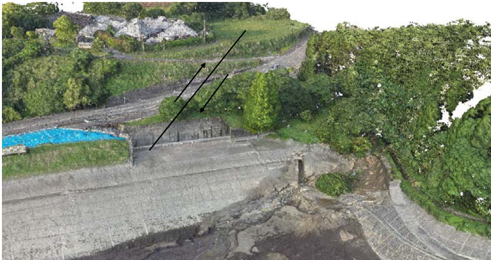
Fig.5 Three-dimensional (3D) model of the spillway generated by UAV data.
