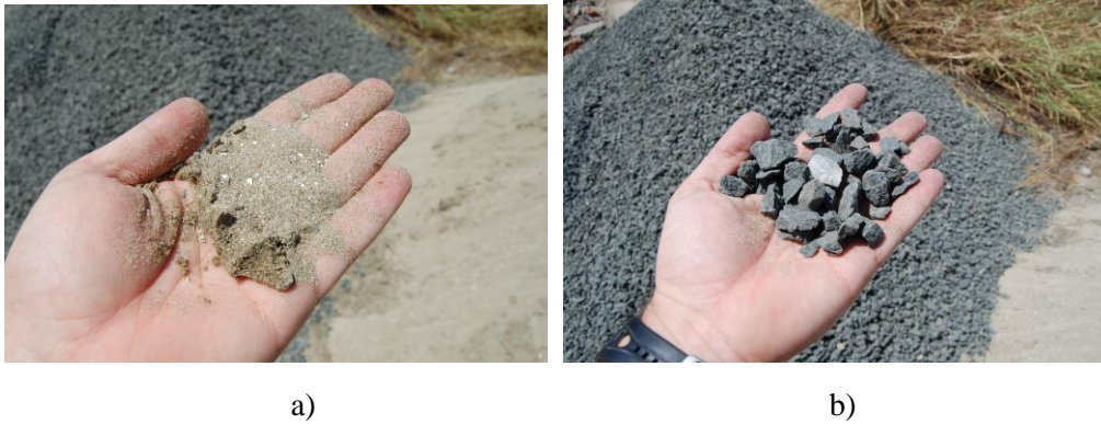
Fig. 22: Building materials near Los Esteros Market in Tarqui, Manta. a) Fine aggregate with sea shells. b) Good quality coarse aggregate (GPS coordinates: 0°57'8.94"S, 80°42'29.38"W). (Photos by C. Arteta Torrents)
