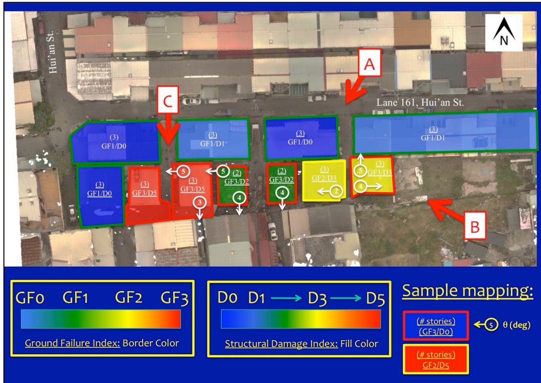
Fig. 7 – Assessment of ground failure – structural damage index (A, B, C denote images shown in Figures 8, 9, and 10 respectively). (center of region at: 23.0254°, 120.2074°)
