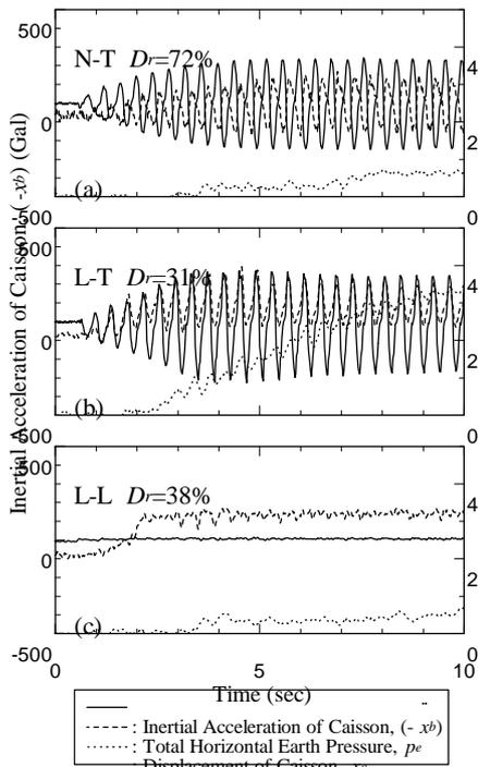
**Figures 3(a-c): Time histories of acceleration, earth pressure and displacement measured in; (a) Case N-T, (b) Case L-T, (c) Case L-L.**
