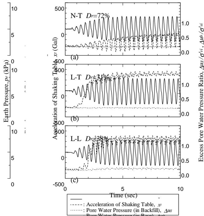
**Figures 4(a-c): Time histories of acceleration and pore water pressure in backfill measured in the test. (a) Case N-T, (b) Case L-T, (c) Case L-L.**
