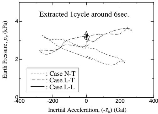
**Figure 7: Relationship between earth pressure and inertial acceleration**
