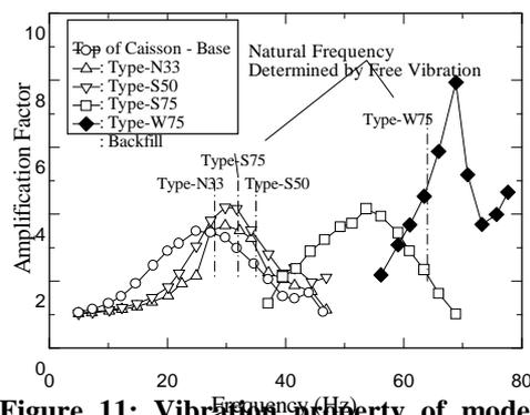
Figure 11: Vibration property of model quay wall
