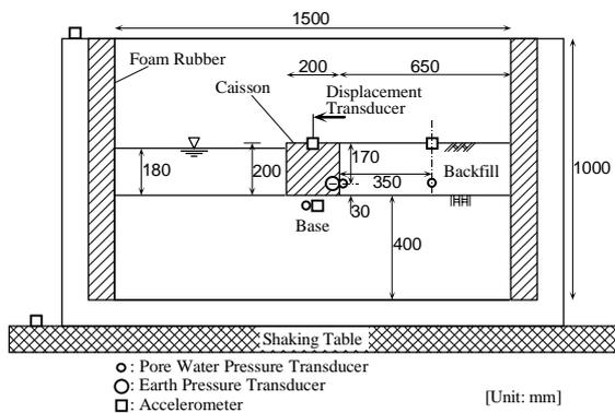
Figure 1(b): Arrangement of measurement devices
