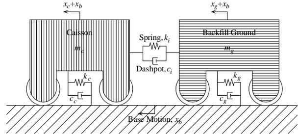
Figure 12: Mass-spring-dashpot model
