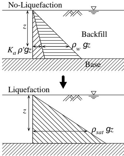
**Figure 5: Static increase in earth pressure due to reduction in effective stress by liquefaction**
