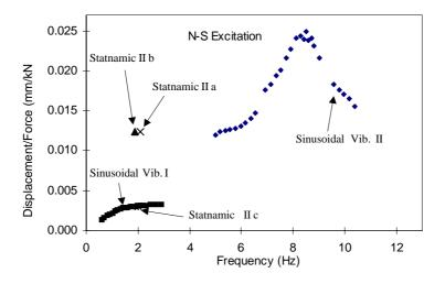
Figure 2. Displacement per unit force from sinusoidal vibration and statnamic II
