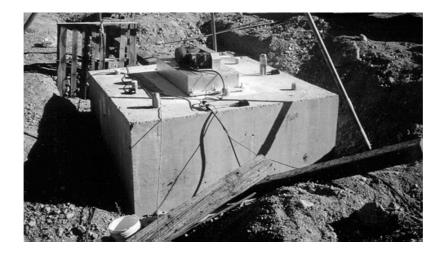
Figure 5. Pile cap and eccentric mass shaker
