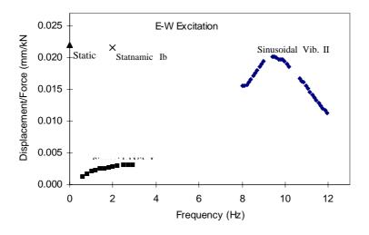
Figure 3. Displacement per unit force from sinusoidal vibration, static, and statnamic I
