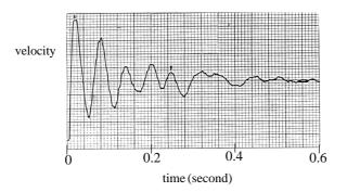
Figure 4. Velocity recorded on strip chart for the N-S impact vibration test
