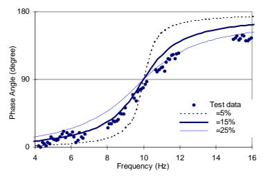
Figure 6. Phase angle versus frequency E-W excitation sinusoidal vibration II
