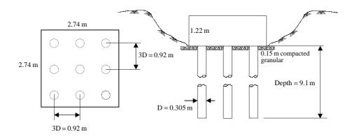
Figure 1. Dimension of the pile group
