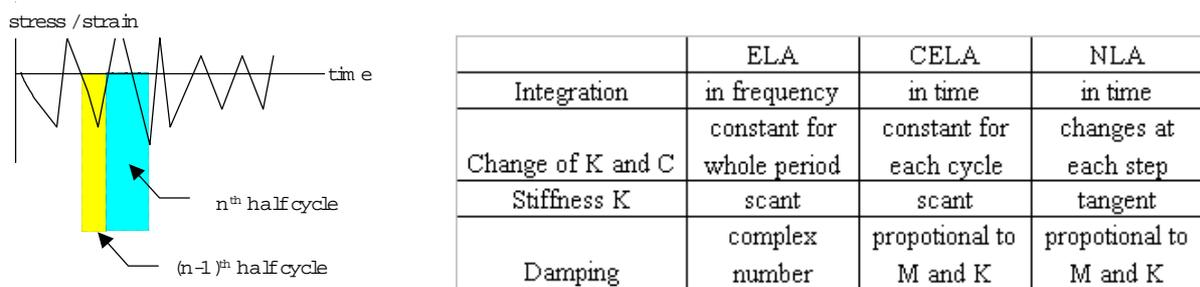
**Figure 3: Concept of Cycle-wise Equivalent Linear Method**
