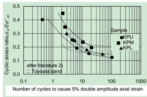
**Figure 4: Liquefaction strength**
