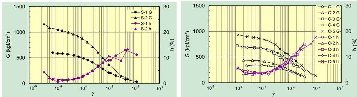
**Figure 5: Scant shear modula for soil layers**
