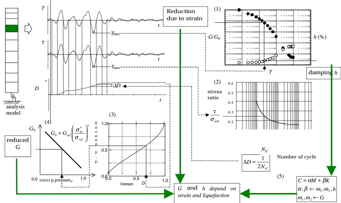
**Figure 7: Concept of cycle-wise equivalent linear analysis for liquefaction**
