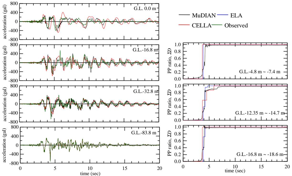
**Figure 9: Liquefaction Simulation of Port Island (Time history of acceleration and excess pore pressure ratio / accumulated damage ratio)**
