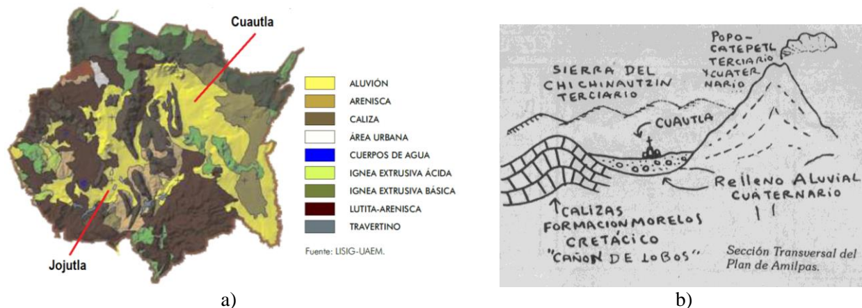
Fig. 12 – a) Location of Jojutla and Cuautla over alluvial soil deposits ( aluvión ) [9], and b) Geological cross section of Cuautla indicating alluvial soil deposits underneath [10]
