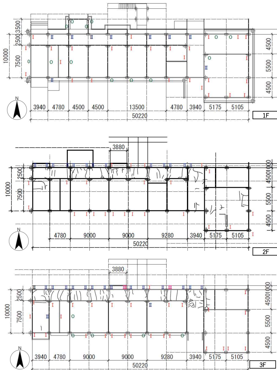
Figure.3 Post-earthquake damage evaluation for the beams and floor slabs
