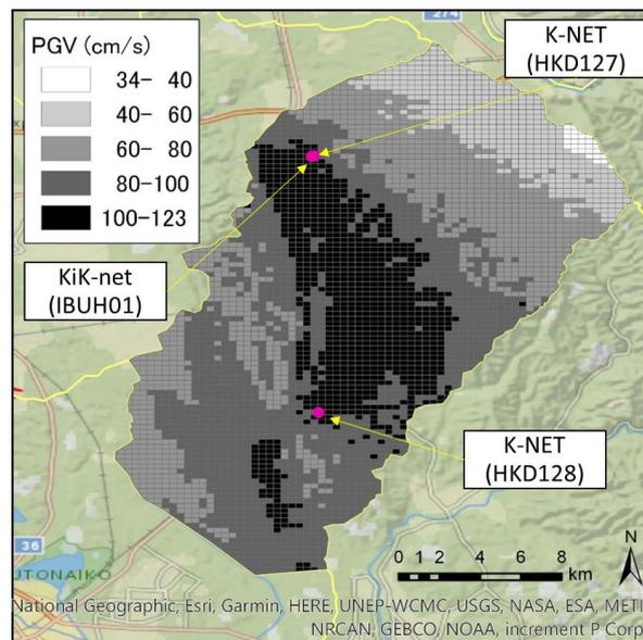
Fig. 3 – Estimated peak ground velocity (PGV) distribution in 250-m grid in Abira Town
