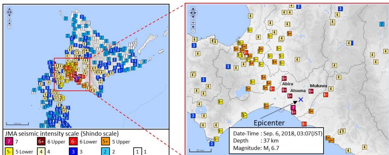
Fig. 1 – Map of JMA seismic intensity on the 2018 Hokkaido Eastern Iburi earthquake (Source: JMA)
