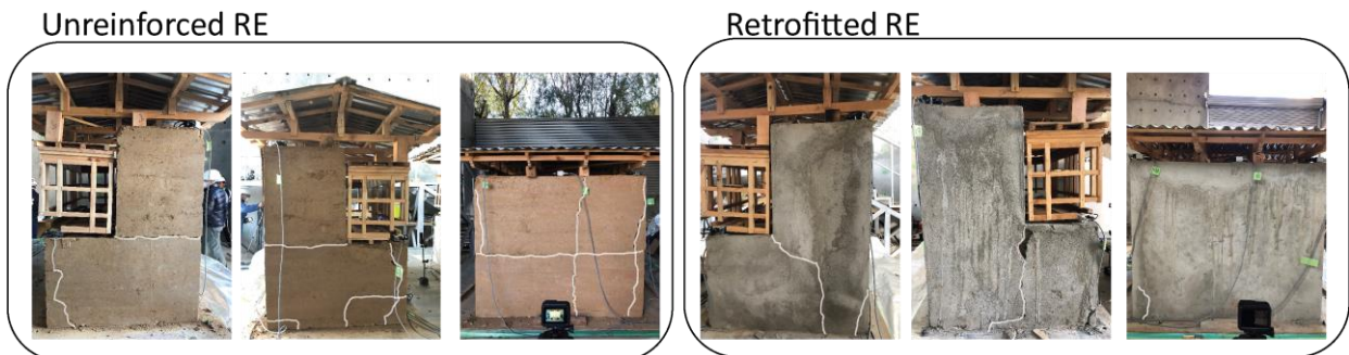
Fig. 13 – Damage for unreinforced and retrofitted specimens at PGA 1.0g.
