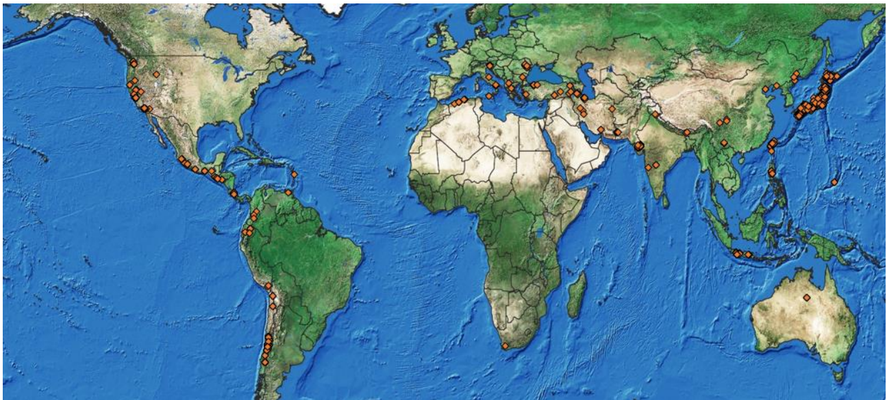
Fig. 10 – Locations of the dams with an evaluated seismic feedback higher than 0.2 g
