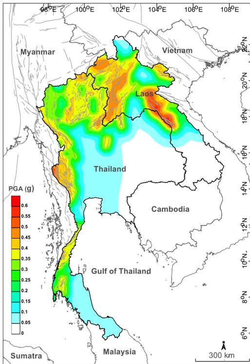
Fig. 2 -Deterministic seismic hazard analysis (DSHA) map of Thailand and Laos showing distribution of peak ground acceleration (PGA) in g.
