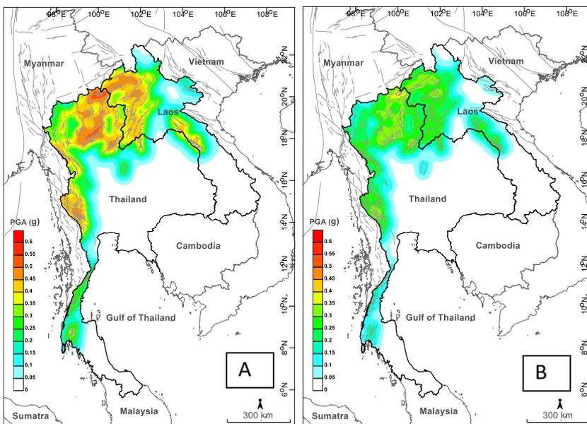
Fig. 4. Probabilistic seismic hazard analysis (PSHA) maps of Thailand and Laos illustrating the PGA distribution with (a) 2% POE within the next 50 yr and (b) 10% POE within the next 50 yr
