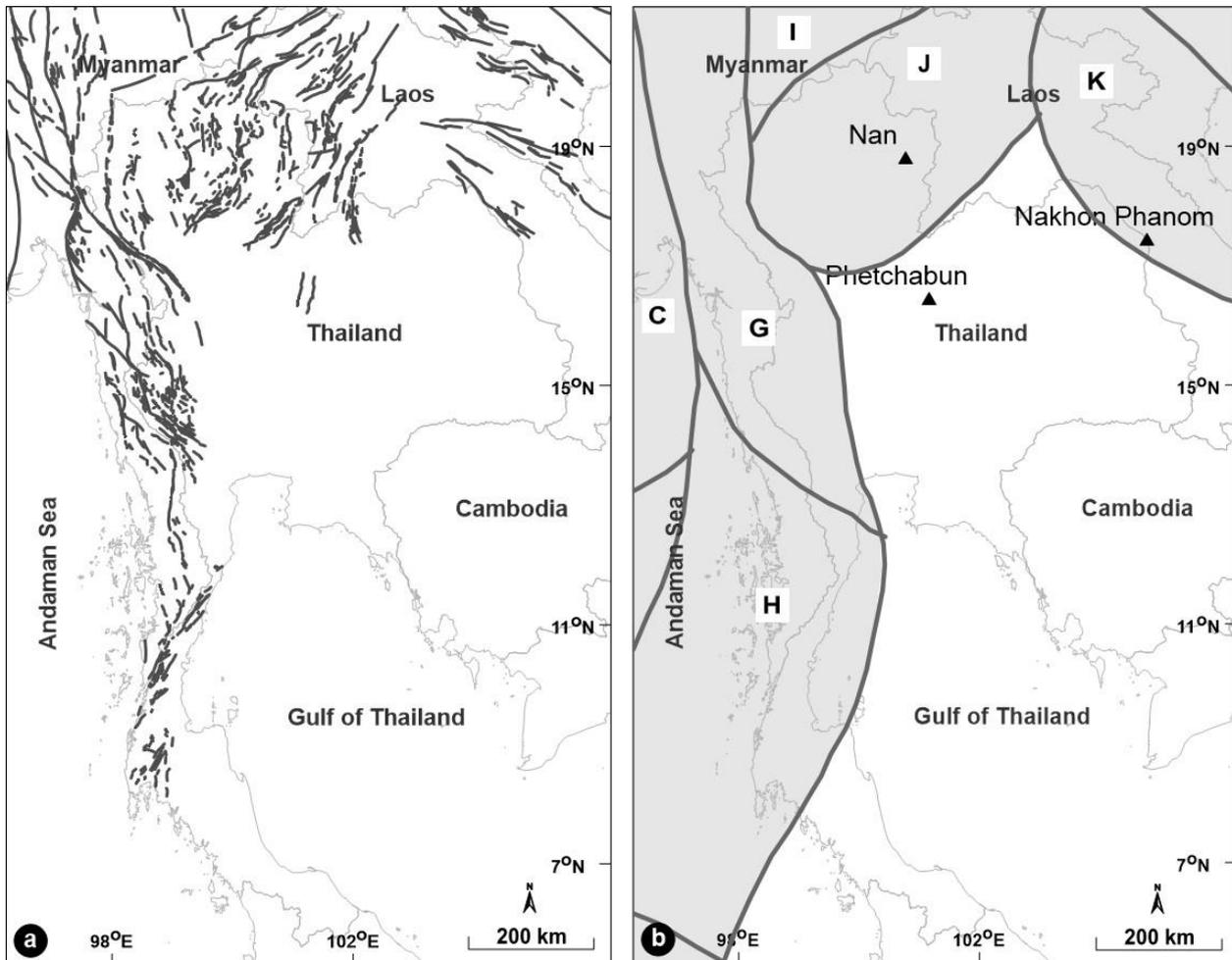
Fig. 1 -Map of Thailand and the neighboring areas illustrating (a) the possible active fault lines or lineaments and (b) seismic source zones covering Thailand and Laos, as proposed by Pailoplee and Choowong [9]. The black triangles are the new sites of paleoseismological investigations used in this study.
