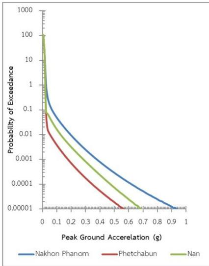
Fig. 3-Hazard curves showing relationship of peak ground acceleration (PGA) and probability of exceedance (POE) for 3 new locations where active faults have been recently recognized. Their geographical locations are shown in Fig. 1b.
