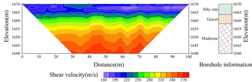
Fig. 7 Shear velocity profile of surface wave test and borehole information
