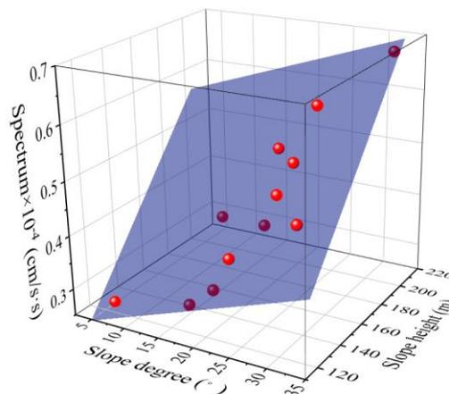
Fig. 9 Relation between slope degree, height and spectrum amplitude
