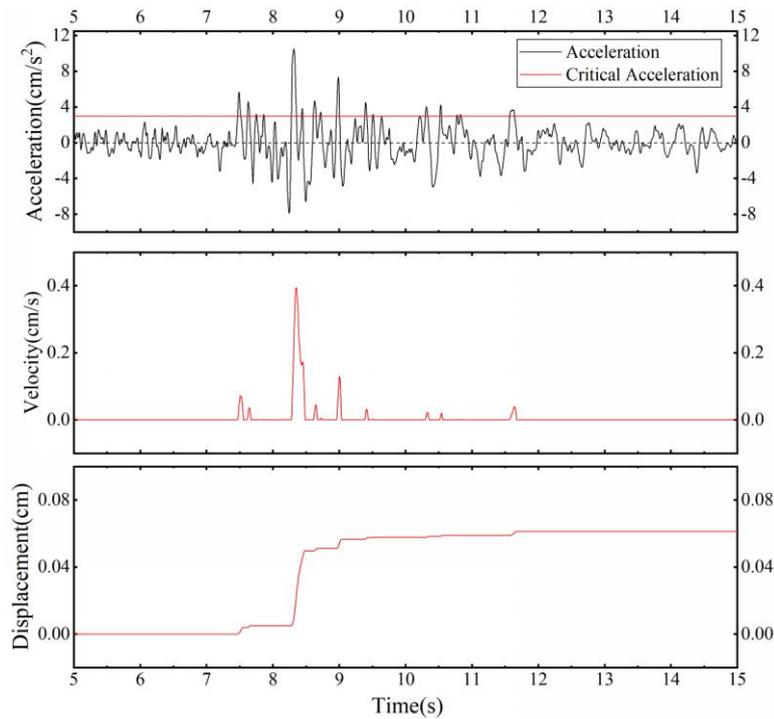
Fig. 2 Sketch of two-stage integration process in Newmark model
