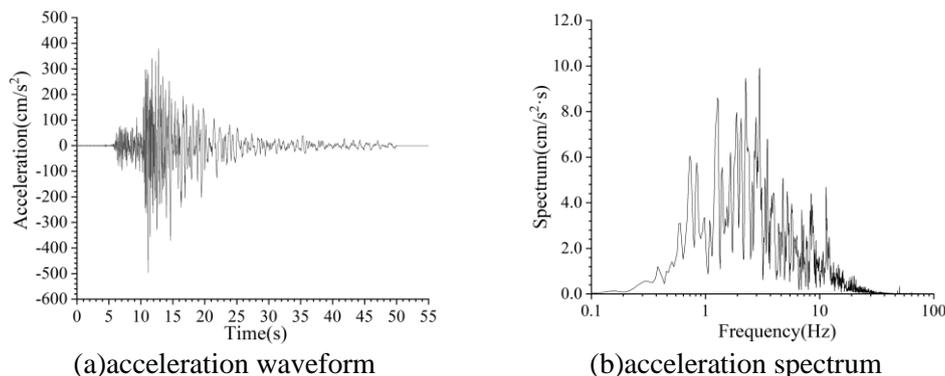
Fig. 8 Acceleration wave and spectrum (recorded at Chenghai observation station under 2019 Yongsheng earthquake)
