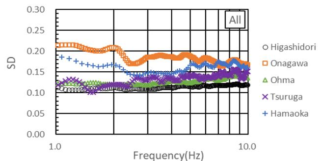
Fig.10 Relationship between SD of H/V spectral ratio and frequency.
