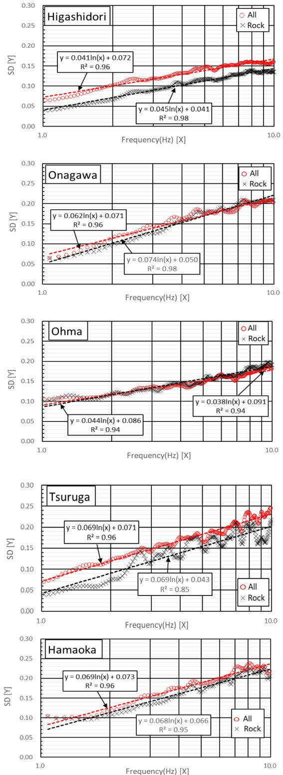
Fig.6 Relationship between the SD and frequency of “All” and “Rock” at each site.
