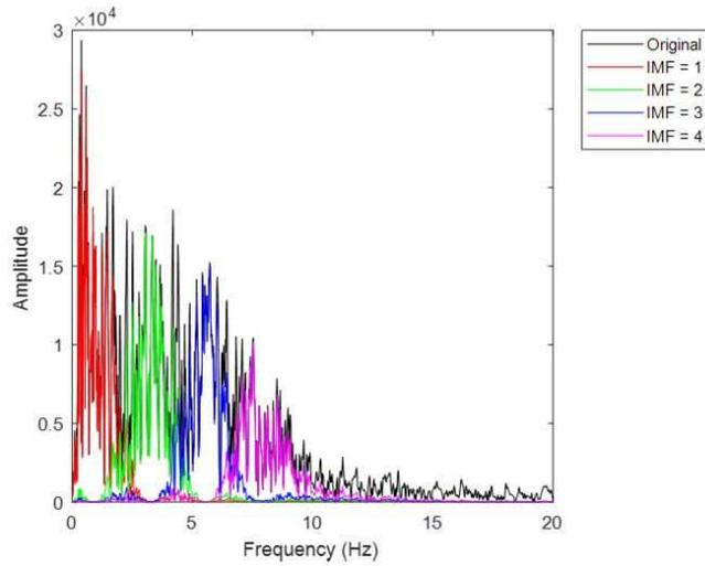
Fig. 4 – Fourier amplitude spectrum of the AMNT –EW component- original signal and comparison with the FFT based spectra of the decomposed signal (for the four IMF sequences considered). Noise reduction effect in the decomposed modes can be appreciated
