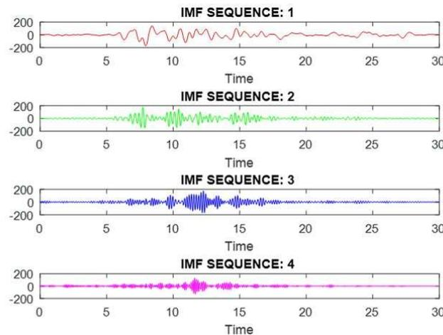
Fig. 3 – VMD results of the AMNT record showing IMF modes with less noise contamination, especially in sequences 2, 3 and 4
