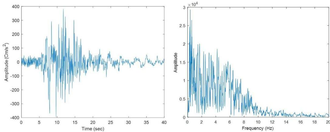
Fig. 2 – AMNT record -EW component- and Fourier amplitude spectrum of the signal
