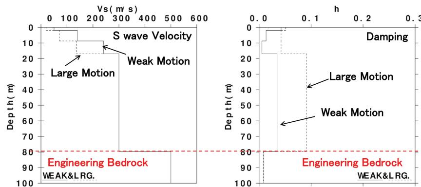
Fig. 4 – Difference of shallow S wave velocity and damping models under weak and large motions.
