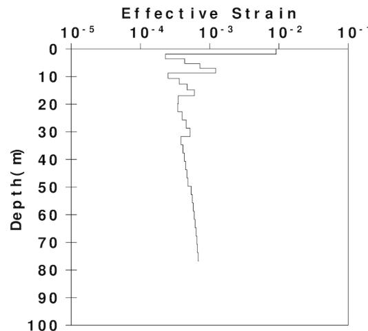
Fig. 10 – Depth distribution of effective strain in calculation of Fig. 7
