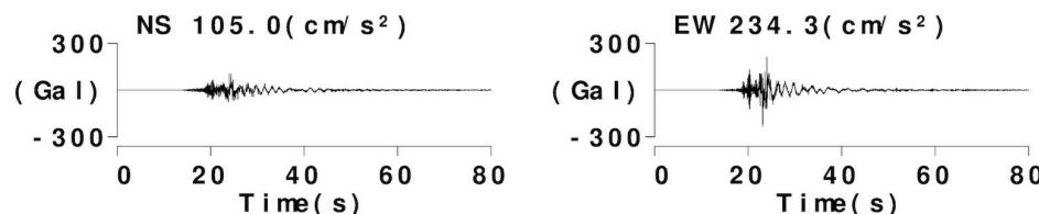
Fig. 6 – Estimated input ground motion of the 2000 western Tottori prefecture earthquake on engineering bedrock at JMA Sakaiminato site (Free surface)
