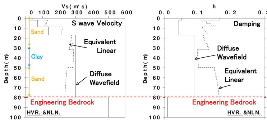
Fig. 9 – Comparison of estimated S wave velocity and damping structured between diffuse wavefield theory (solid line) and equivalent linear analysis (dash line)
