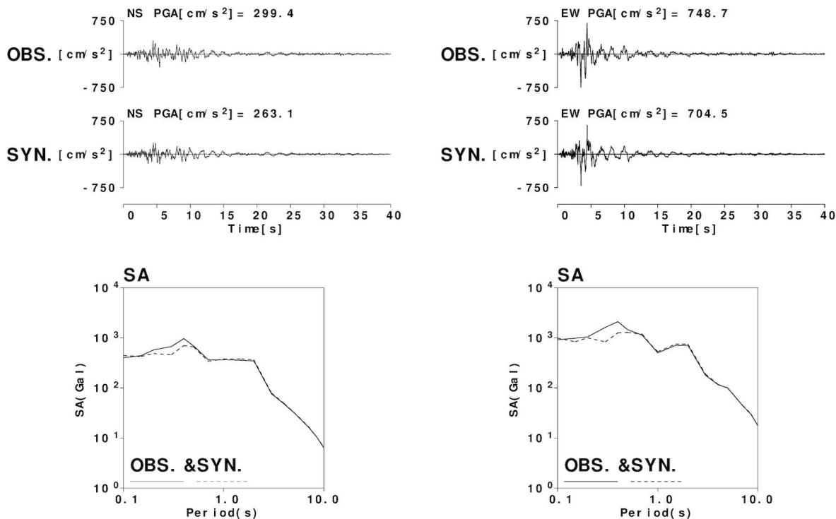
Fig. 7 – Comparison between observed and synthesized waves
