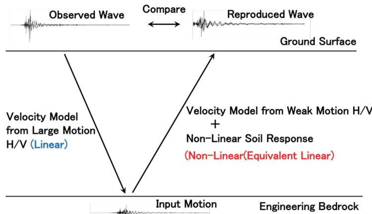
Fig. 5 – Schematic diagram of analysis method in this study
