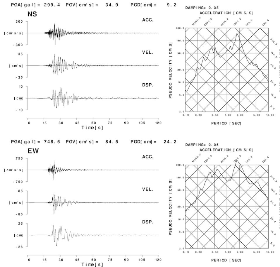
Fig. 1 – Main shock observation record at the JMA Sakaiminato site due to the 2000 western Tottori prefecture earthquake (Acceleration, velocity, displacement waveform of two horizontal components and their tripartite response spectra)
