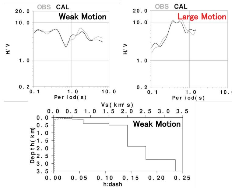
Fig. 3 – Observed and synthesized H/V spectra of weak motion (upper left) and large motion (upper right) with velocity structure model down to the seismic bedrock in case of weak motion.
