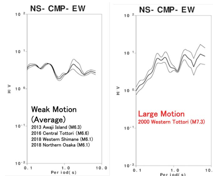
Fig. 2 – H/V spectra of weak motions and large motion at the JMA Sakaiminato site
