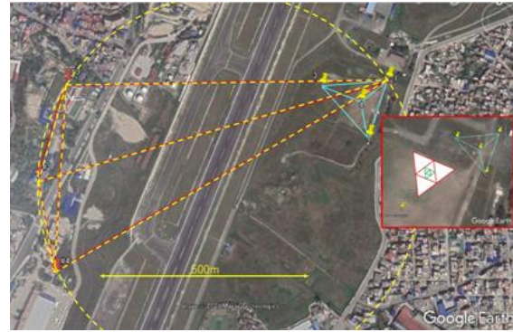
Fig.5a TIA (Tribhuvan International Airport): Configuration of Arrays deployed (after Google Earth®). Solid yellow segment denotes 500 m.
