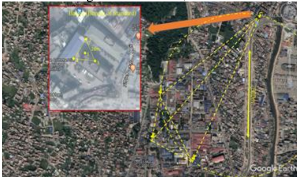
Fig.11a BLJ (Balaju Industrial District): Configuration of deployed arrays (after Google Earth®). Solid yellow segment denotes 500 m.
