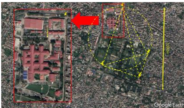
Fig.7a CHH (Chhauni Army Barrack – Hospital): Configuration of deployed arrays (after Google Earth®). Solid yellow segment denotes 1,000 m.
