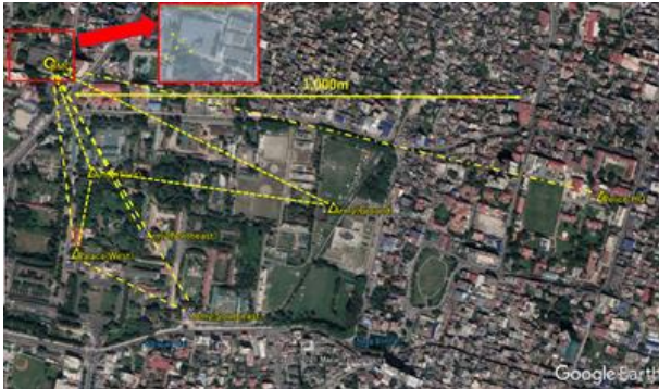
Fig.12a DMG (DMG-Narayanhiti): Configuration of deployed arrays (after Google Earth®). Solid yellow segment denotes 1,000 m.
