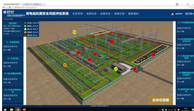
Fig. 12 Damage evaluation of subparts in a substation
