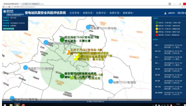
Fig. 11 Seismic assessment of substations in a region
