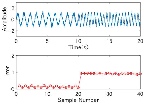
Fig.5 Change of frequency with noise
