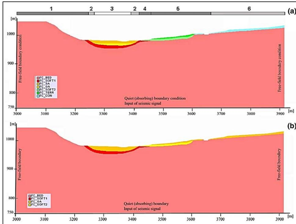
Fig. 2 - Seismo-stratigraphic layering (see Table 2) of HeM (a) and HoM (b) models; for HeM the positions of the defined microzones (from 1 to 6) are also indicated in the upper bar
