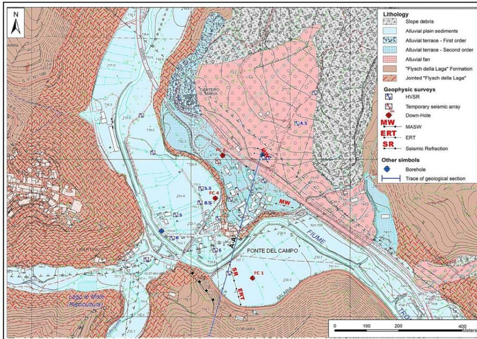
Fig. 1 - Lithotechnical map of Fonte del Campo (Accumoli). The trace of the AA' geological cross section of Fig. 2 is also reported
