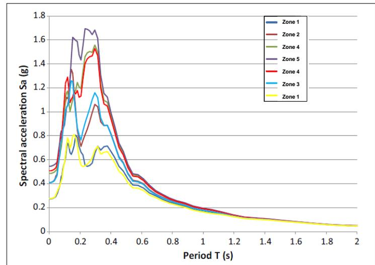
Fig. 6 - Ground acceleration response spectra for each zone (Z1-Z2-Z4-Z5-Z4-Z3-Z1) defined in SM3 map
