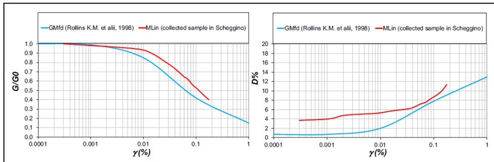
Fig. 4 - Normalized shear modulus  $G/G_0$  and damping ratio  $D$  versus shear strain  $\gamma$  curves for the main lithotechnical units
