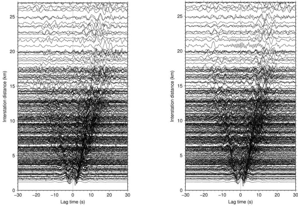
Fig. 3 – Crosscorrelation functions of the vertical component (left) and the transverse component (right).
