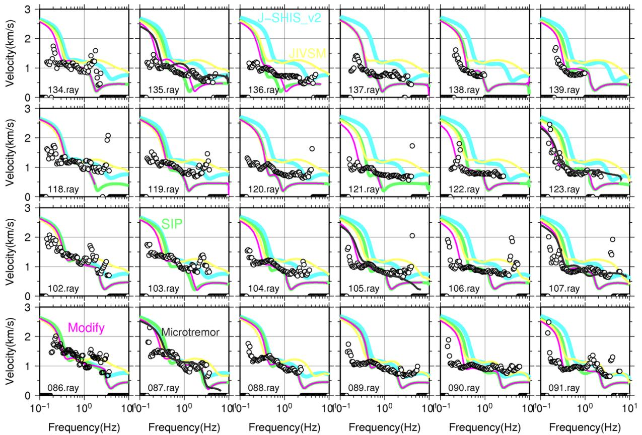
Fig. 8 – Comparison of the dispersion curves among observed and theoretical group velocity of fundamental mode of Rayleigh wave. These cells are corresponding to Fig. 6.
