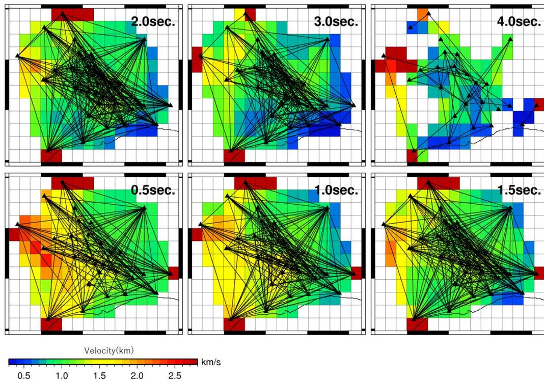
Fig. 5 – Group velocity of Love wave at the periods from 0.5 to 4.0 seconds calculated by the tomographic analysis.
