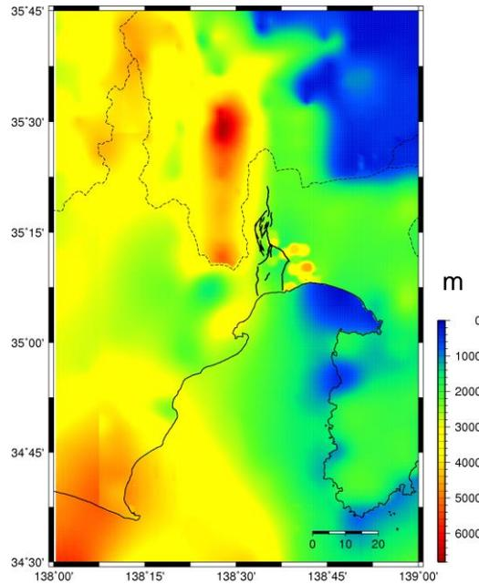
Fig. 7 – Depth to the seismic bedrock with the  $V_s$  of 3.2 km/s.
