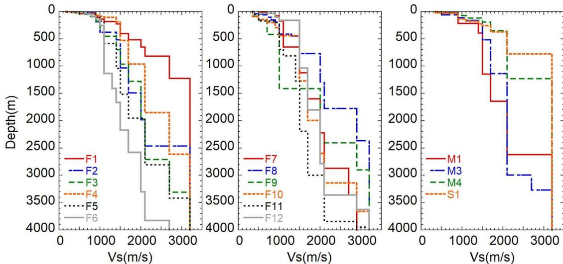
Fig. 2 – S-wave velocity structure model estimated by inversion of dispersion curve.
