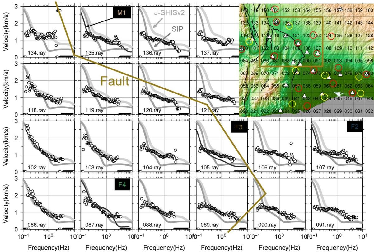
Fig. 6 – Dispersion curve of group velocity at the cells shown by rectangular in the top right panel. Circle indicates the estimated group velocity of Love wave by tomographic analysis. Gray line shows the theoretical dispersion curve of Love wave group velocity calculated using the J-SHIS [3] (light gray) and Wakai et al. (2019) [8] (gray). Black is theoretical dispersion curve for the model estimated by array microtremor exploration.
