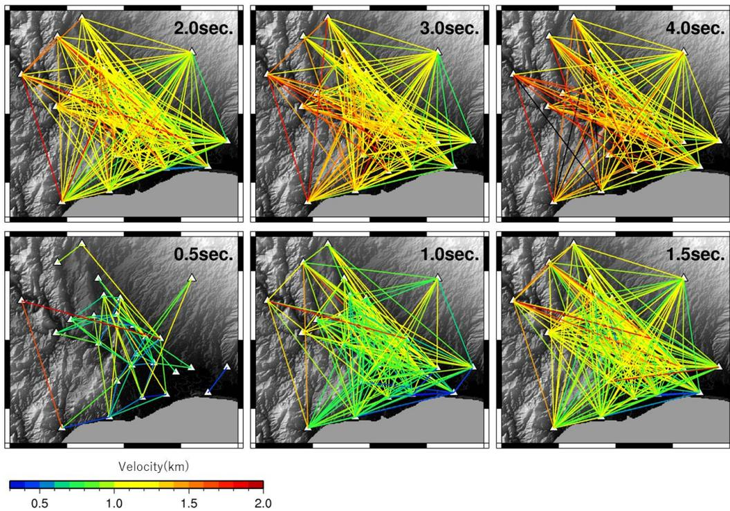
Fig. 4 – Distribution of group velocity of Love wave at the periods from 0.5 to 4.0 seconds observed from multiple filter analysis of the crosscorrelation function of the transverse component.
