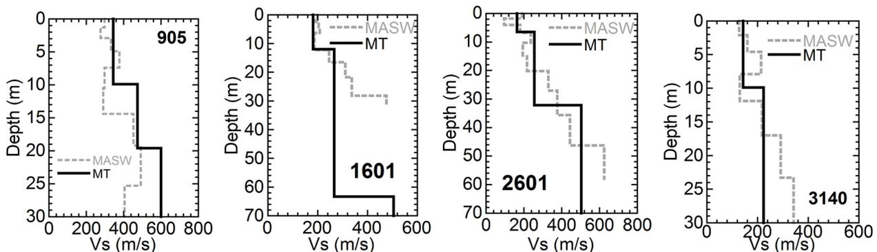
Fig. 8 – Comparison of  $V_s$  profiles between this study and MASW.
