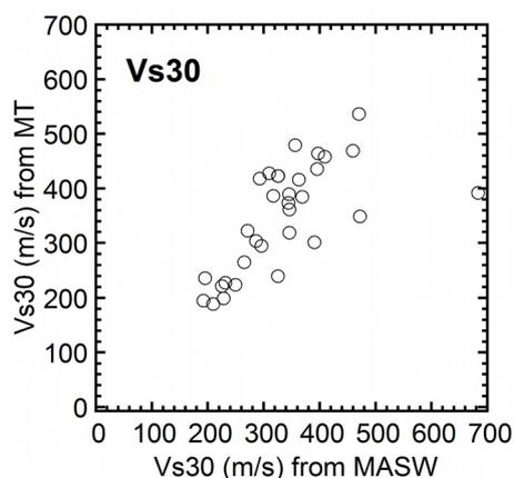
Fig. 9 – Comparison of Vs30s from microtremor explorations in this study (MT) and surface wave explorations compiled by AFAD (MASW).
