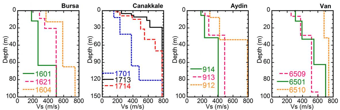
Fig. 7 – Shear-wave velocity profiles derived from phase velocities in Fig.6.
