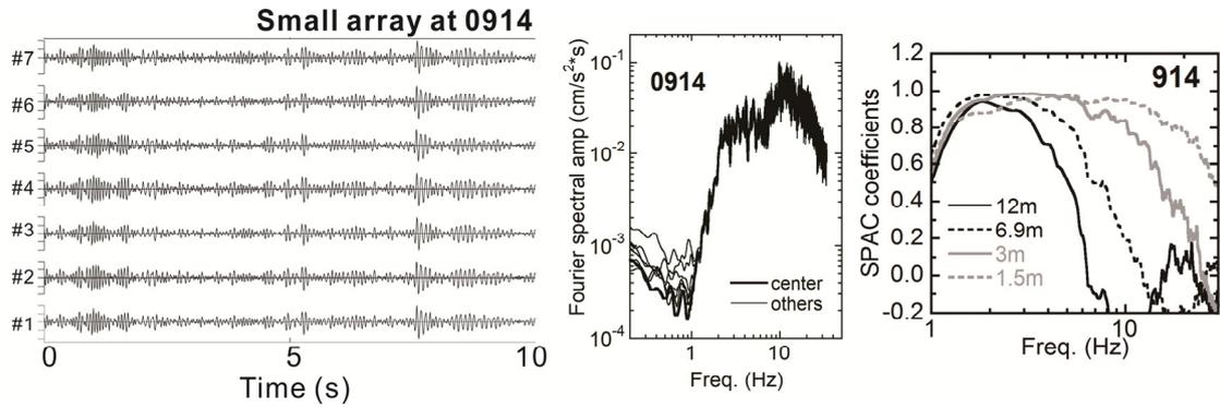
Fig. 5 – Examples of results of SPAC analysis of microtremor array data.
