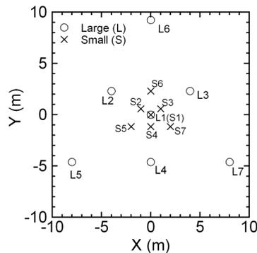
Fig. 4 – Example of array configuration in microtremor exploration
