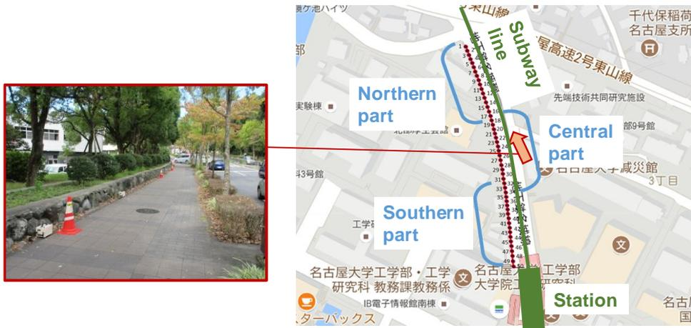
Fig. 1 – Sensor placement for the measurement of the subway train induced vibration
