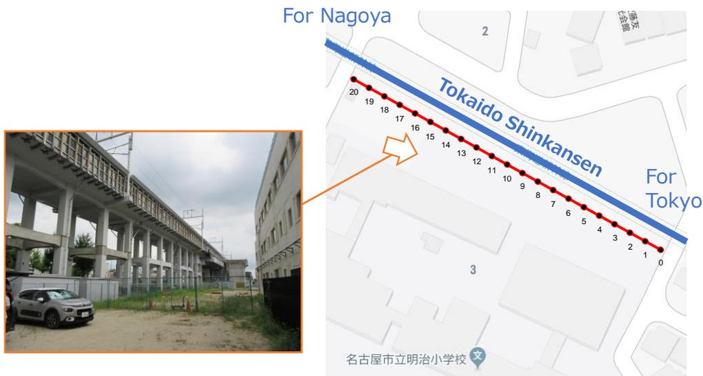
Fig. 2 – Sensor placement for the measurement of the Shinkansen train induced vibration
